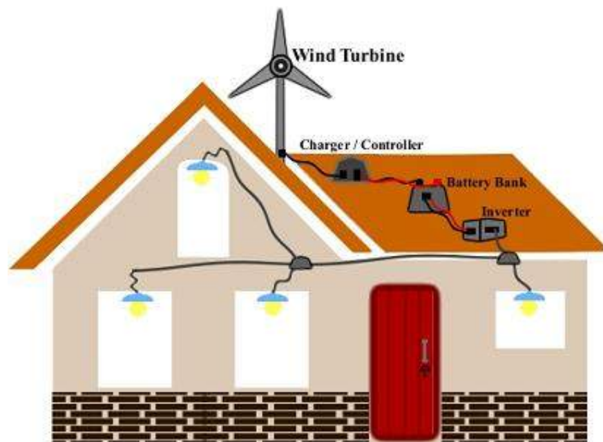
Figure 4.3 Wind Energy System
