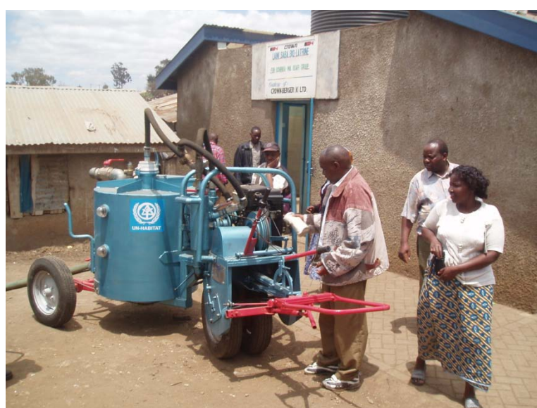
Figure 3.9: The 'vacutug' developed by UN-Habitat.
