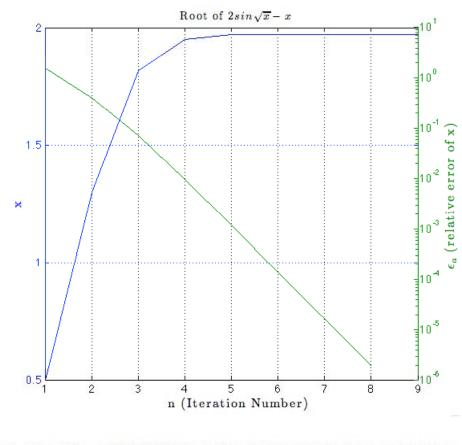
Final Solution: f(x = +1.9723804860817313) = +4.516657e - 07 with Fixed Point method and 8 iterations
