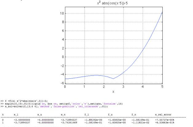
Final Solution: f(x = +3.7434146926188117) = -1.118214e - 02 with FALSE-POSITION method and 1 iterations >> x\_sol=solver(f,[3.4 4],'method','false-position','rel\_tolerance',.001);
