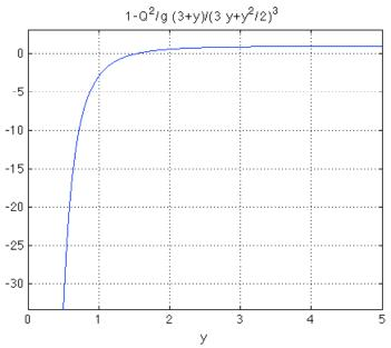
By zooming in the graph we can see that root is approximated by y=1.51 (m). Note as it can be seen the function has considerable curvature around the root. On the other hand (0.5+2.5)/2=1.5 is very
