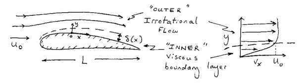
The boundary layer thickness grows with x but is small with respect to the length scale of the surface  $\delta(x)/L \ll 1$ . We proceed as follows:
