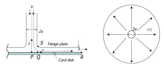
The point *P* is a stagnation point. To find the net pressure force on the disk we need to evaluate the pressure distribution p(r) along the streamline  $\overline{PQR}$ . Model the flow along  $\overline{PQR}$  as inviscid with streamlines that are purely radial with  $v_r = f(r)$ .
