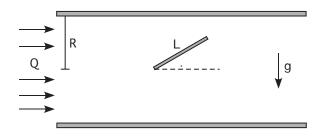
Consider a channel of height 2R with rectangular cross-section as shown in the sketch. A hinged plank of a length L < R and at an angle  $\theta$  is located at the center of the channel. (You may assume that L is small compared to the length perpendicular to the sketch.) The plank has a mass per unit width, m. A constant volume flux per unit width, Q, of an inviscid, incompressible fluid is applied at the inlet of the channel.
