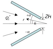
We now consider a simplified geometry to model the first process shown above; i.e. the converging flow of the <u>inner fluid</u> confined between two solid walls inclined at angles  $\pm \alpha$  to the horizontal. We\_will model this flow as a <u>planar two dimensional</u> flow. Use a cylindrical polar coordinate system  $\{r, \theta\}$  as shown in the sketch. For distances  $r \ge H/\sin \alpha$  the flow is purely radial.
