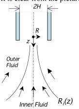
the inner fluid. If we use a <u>cylindrical coordinate</u> <u>system</u> as shown in the sketch opposite then the equation for the interface is  $R_i = Kz^{3/2}$  where K is a constant. Use a lubrication analysis to find the velocity field in the inner fluid, assuming the outer fluid has negligible viscosity ( $\mu_o = 0$ ). Clearly state any assumptions that you make in your solution
