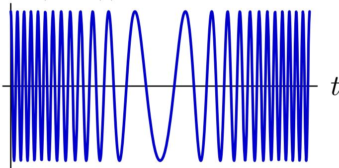
FM generates a very redundant signal, which is resilient to additive noise.
