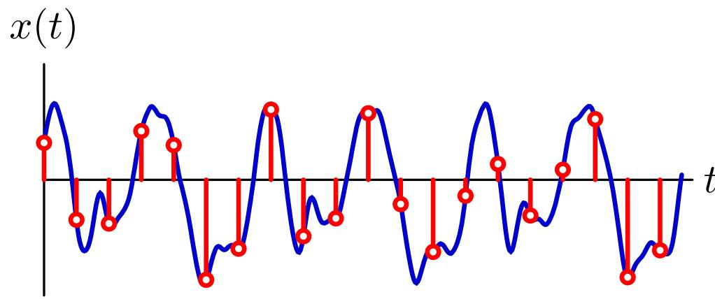
Information between samples is lost. Therefore, the same samples can represent multiple signals.
