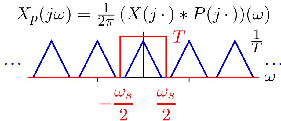
Impulse reconstruction followed by ideal low-pass filtering is called **bandlimited reconstruction**.
