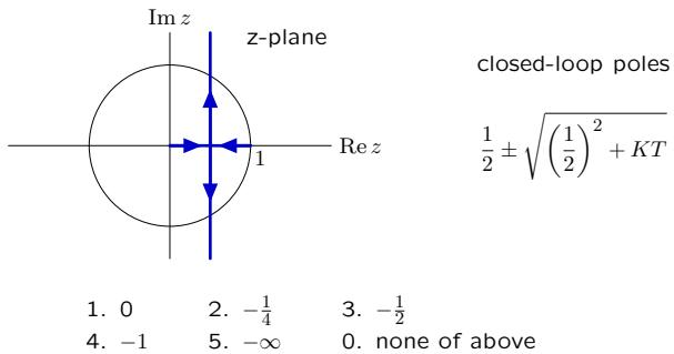
**Destabilizing Effect of Delay**
