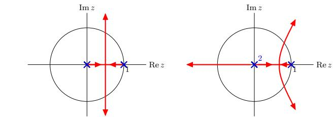
Fastest response with delay: double pole at  $z = \frac{1}{2}$ .
