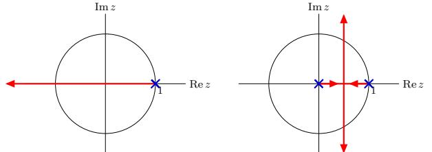
Fastest response without delay: single pole at  $z = 0$ .
