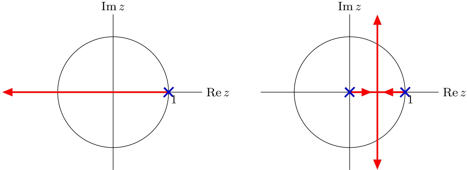
Fastest response without delay: single pole at  $z = 0$ .
