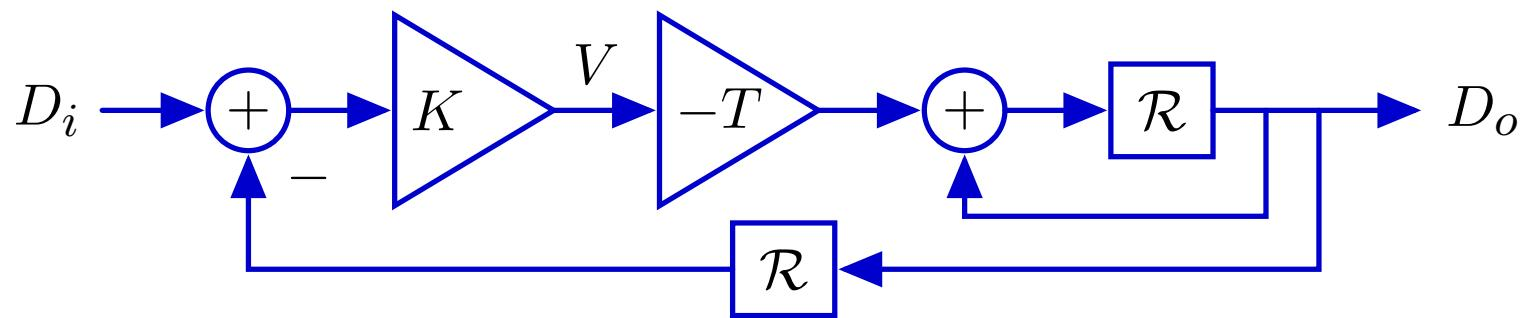
Replace accumulator with equivalent block diagram.
