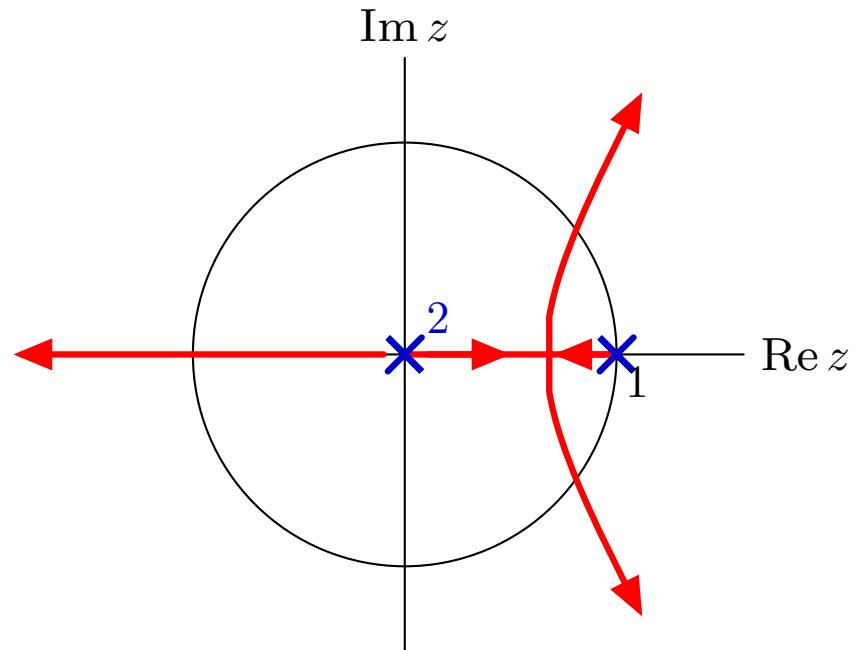
Fastest response with delay: double pole at  $z = \frac{1}{2}$ .
