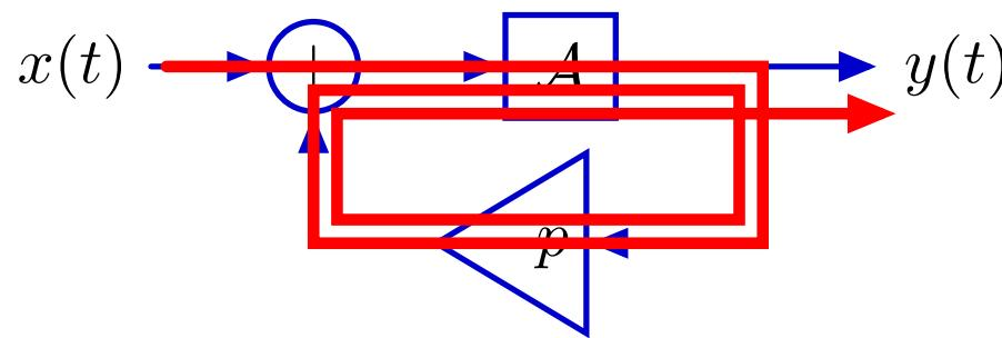
$$\begin{aligned}y(t) &= (\mathcal{A} - p\mathcal{A}^2 + \cancel{p^2\mathcal{A}^3} - p^3\mathcal{A}^4 + \dots) \delta(t) \\&= (1 - pt + \frac{1}{2}p^2t^2 - \frac{1}{6}p^3t^3 + \dots) u(t)\end{aligned}$$
