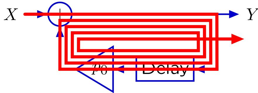
$$\begin{aligned}y[n] &= (1 + p\mathcal{R} + p^2\mathcal{R}^2 + p^3\mathcal{R}^3 + \cancel{p^4\mathcal{R}^4} + \dots) \delta[n] \\&= \delta[n] + p\delta[n - 1] + p^2\delta[n - 2] + p^3\delta[n - 3] + \cancel{p^4\delta[n - 4]} + \dots\end{aligned}$$
