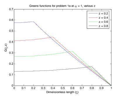
The plot above shows that at a given point source, there is a balance between diffusion and firstorder consumption satisfying both boundary condition (zero gradient left, G = 0 right). A species right of the source will decrease due to diffusion and consumption to satisfy zeroconcentration at the right boundary. A species left of the source will decrease so that the no flux condition is satisfied at the left.
