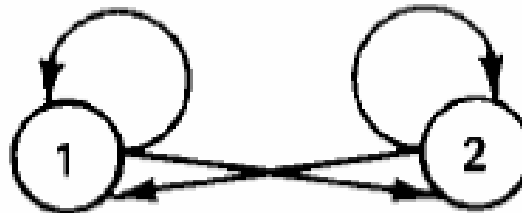
a. Example of a state diagram with N=2 states
