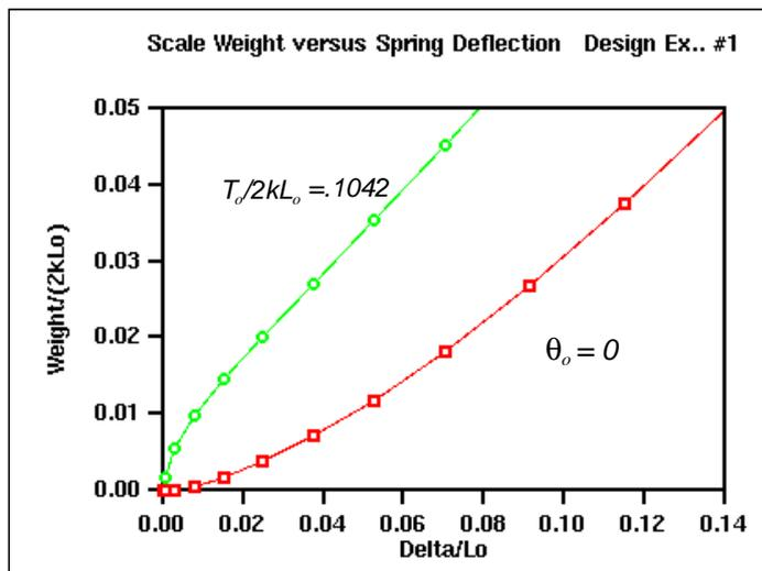
The effect of the pretension is two - fold: A bigger weight is required to move the pointer to the same position (as that taken up by a system with  $\theta_0 = 0$  and no pre-tension) and the graph appears to become linear earlier on, at a lower weight.
