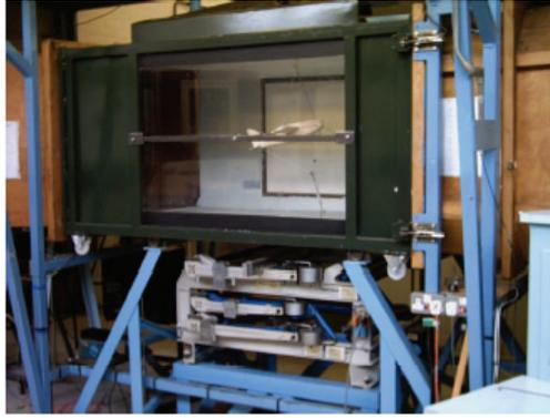
Fig. 1. The flexible suspension system for wind tunnel
