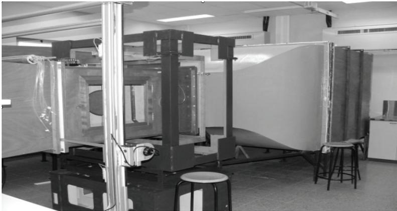
Fig. 1. Wind tunnel device in the aerodynamic laboratory of BGU of the Negev, (general view).
