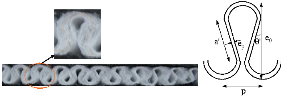
Fig. 16. Geometrical modelling of the pleat after the laminating process
