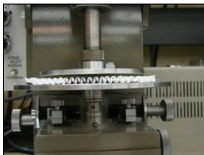
Fig. 20. Customization of the KES-FB3 compression tester
