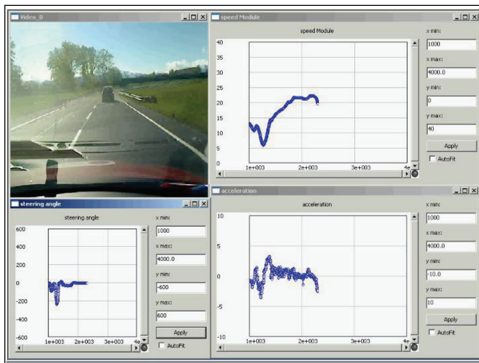
Fig. 9. Video/CAN-bus data visualization
