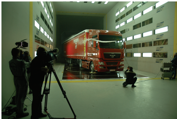
Fig. 7. Truck in 9.5x9.5 test section
