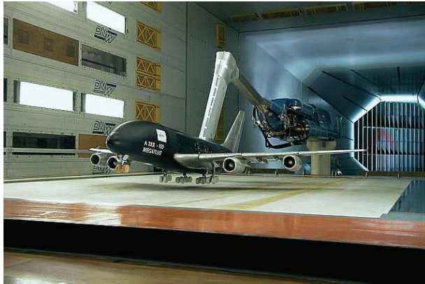
Fig. 6. Model on sting above moving belt
