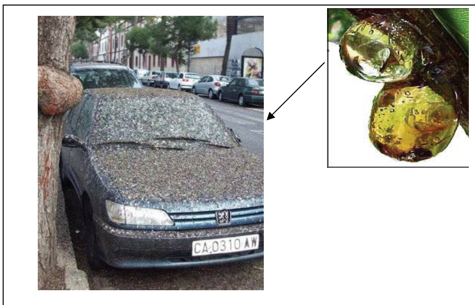
Fig. 19. Effect of Arabic gum on car body.
