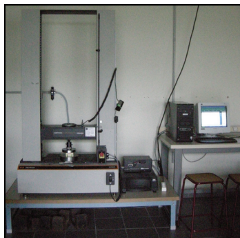
Fig. 21. INSTRON 33R4204 testing device
