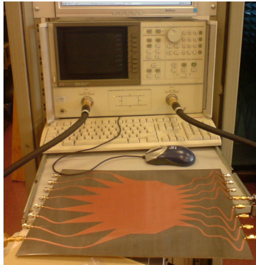
Fig. 6. Fabricated 8×8 ITS Rotman Lens Microwave BFN.
