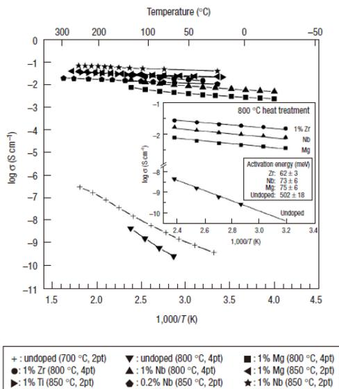
Fig. 7. The electrical conductivity of Doped olivines of stoichiometry  $\text{Li}_{1-x}\text{M}_x\text{FePO}_4$   $\text{M}=\text{Mg}$ ,  $\text{Ti}^{4+}$ ,  $\text{Zr}^{4+}$  and  $\text{Nb}^{5+}$ ) (Chung et al., 2002)
