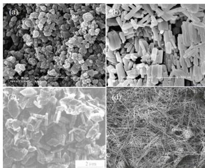
Fig. 11. The SEM micrograph of prepared  $\text{LiFePO}_4$  with various morphologies: (a) Spherical particals(Kima et al., 2007), (b) nanorods(Huang et al., 2010), (c) flaky materials(Zhuang et al., 2005) and (d) nanowires(Wang et al., 2009)
