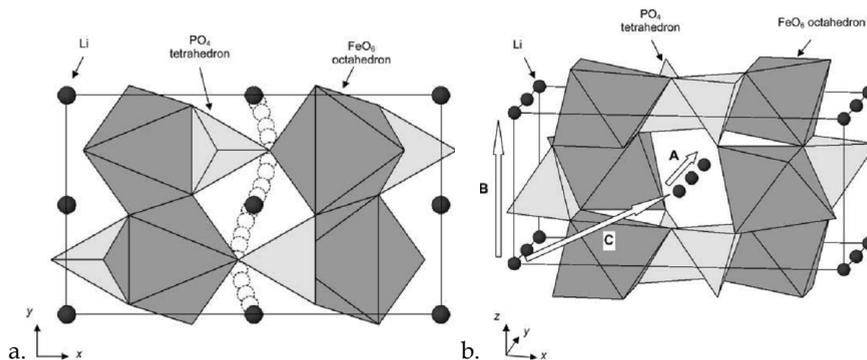
Fig. 5. Curved trajectories for Li ion migration between sites in the [010] direction. The diffusion path lies out of the  $x$ - $y$  plane. (a, 2D model. b, 3D model, A, B, C denote [010], [001], [101] direction respectively)
