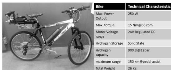
Fig. 19. Hydrogen bicycle and technical characteristics.
