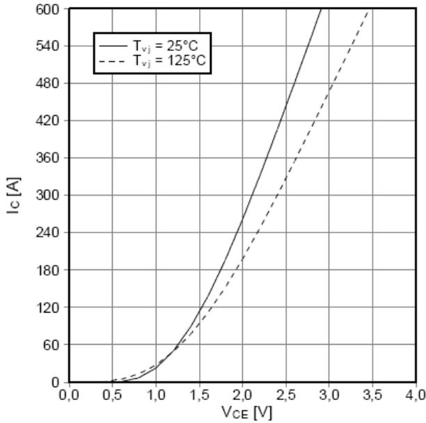
Fig. 10. IGBT BSM300GA120DLC output curve under different voltage
