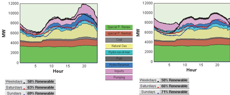
Fig. 18. Example of the expected Winter demand profile for a dry year 2020 in an EVs' peak and off-peak recharge scenario
