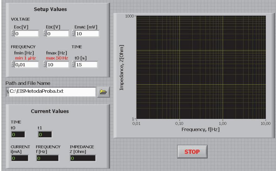
Fig. 3. Front panel of the measuring system for electrochemical impedance spectroscopy
