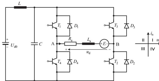
Fig. 8. Transistor bridge
