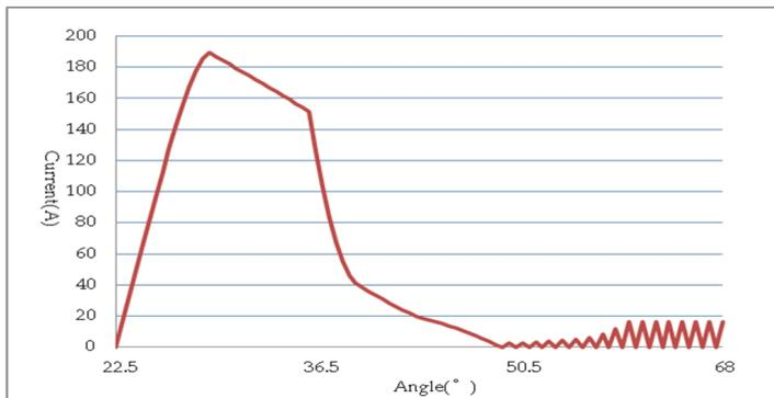
Fig. 3. Profile of designed SRM current vs. angle
