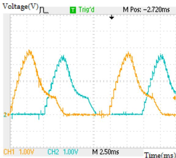
Fig. 19. Winding current waveform of n=500r/min under loaded 72Nm
