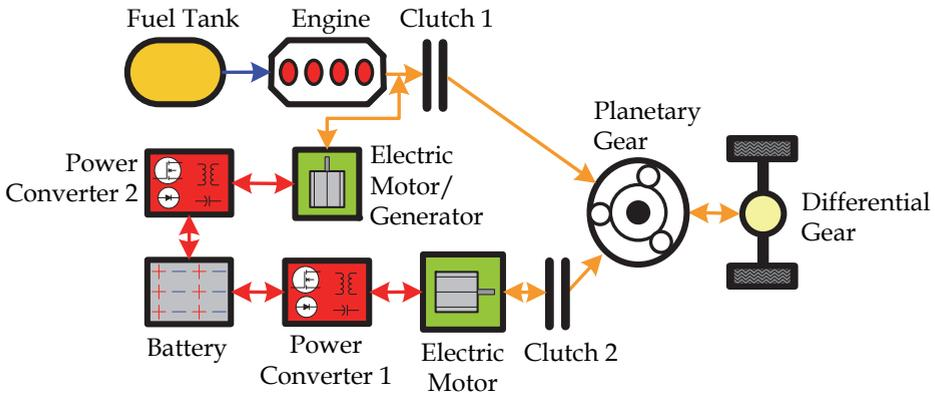
Fig. 12. Architecture of complex HEV
