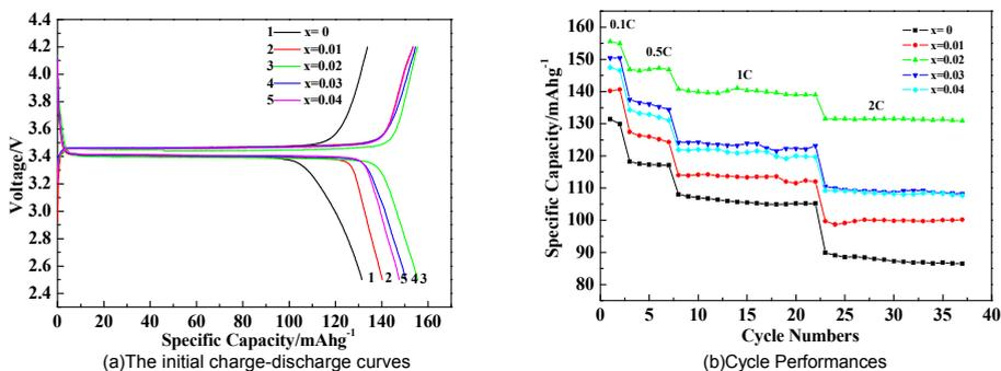
Fig. 8. The electrochemical performances of  $\text{LiFe}(\text{PO}_4)_{1-x/3}\text{F}_x/\text{C}$  ( $x=0, 0.01, 0.02, 0.03, 0.04$ )
