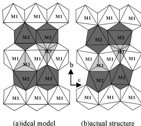
Fig. 2. Crystal structure of LiFePO<sub>4</sub> (a) ideal model and (b) actual structure.
