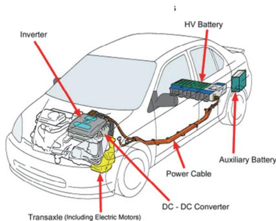
Fig. 14. Power converters in a 2001 Toyota Prius HEV [Automobile Research Bulletin, 2008]
