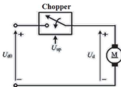
Fig. 7. Simplified presentation of the chopper supply of a DC motor
