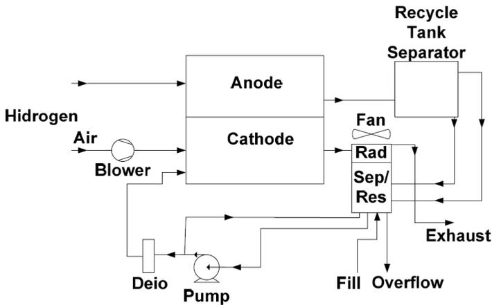
Fig. 22. Schematic diagram of the Fuel Cells System.
