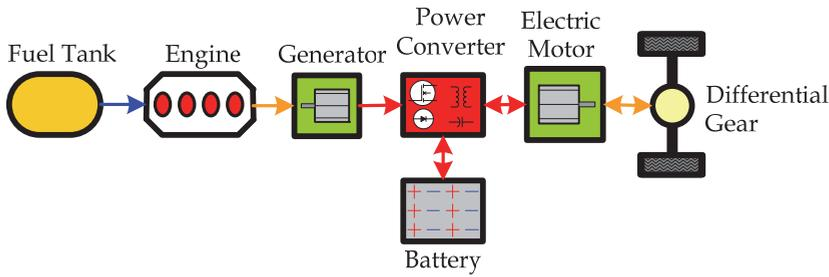
Fig. 8. Architecture of series HEV
