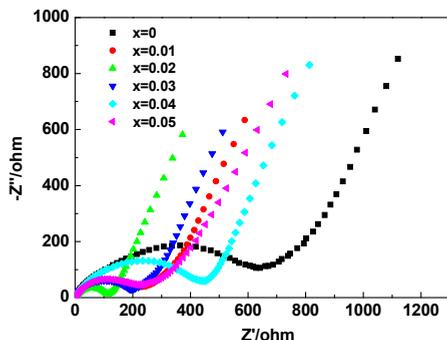
Fig. 9. Electrochemical impedance spectra of LiFe(PO<sub>4</sub>)<sub>1-x/3</sub>F<sub>x</sub>/C (x=0, 0.01, 0.02, 0.03, 0.04) cathodes at 25°C (amplitude is 5mV in the frequency range of 10<sup>5</sup>Hz~0.01Hz)
