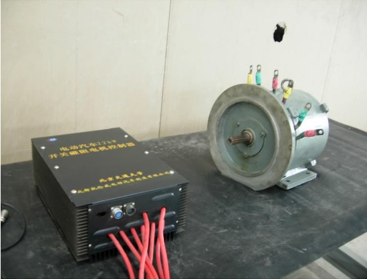
Fig. 23. SR drive system for EV
