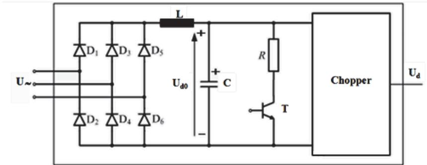
Fig. 6. Principal scheme of chopper supply
