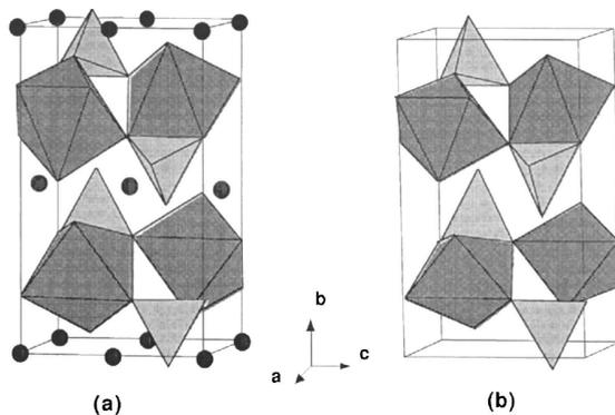
Fig. 3. Crystal structure of (a) LiFePO<sub>4</sub> and (b) FePO<sub>4</sub>
