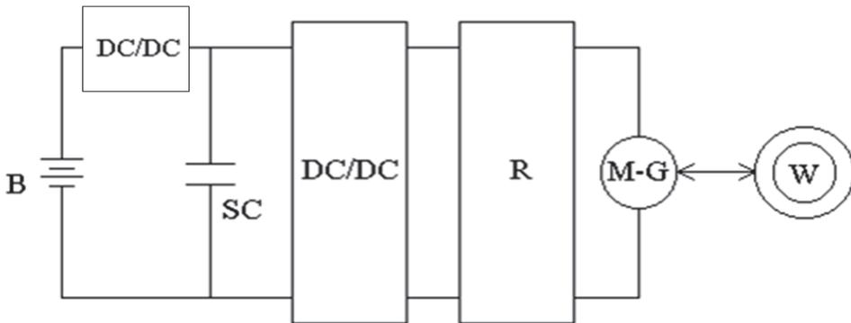
Fig. 5. Scheme of electrical drive vehicle with supercapacitor with possibiltity for using breaking energy; B - one-way voltage source, SC - supercapacitor; DC/DC - direct voltage converter; R - regulator; M-G - engine - generator (depending on working regime; W - drive wheels
