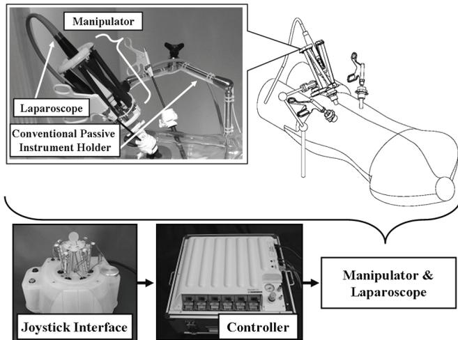
Fig. 5. System configuration
