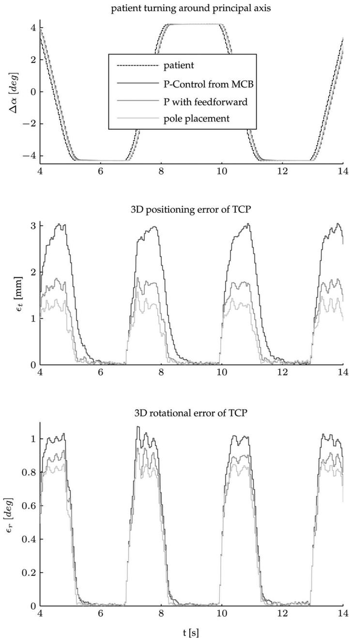
Fig. 10. Comparison of three different control strategies - 1. original proportional controller, 2. proportional with feedforward, 3. pole placement controller
