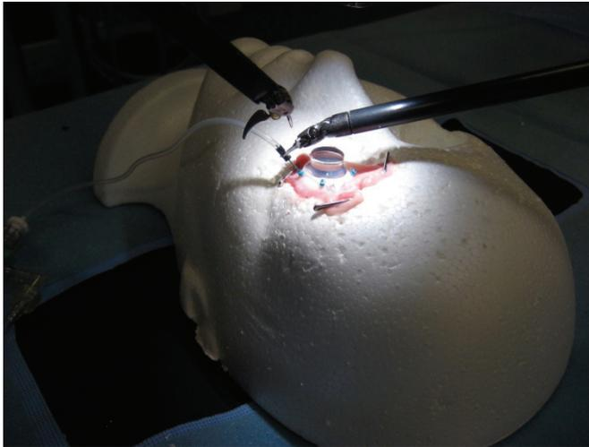
Fig. 7. The *da Vinci* surgical system was used to insert 3 trans-scleral cannulas which is necessary for minimally invasive vitrectomy surgery. In addition to axial motion, the wrist-like tips of the robotic instruments have roll, pitch, yaw and grip to facilitate delicate manipulations.
