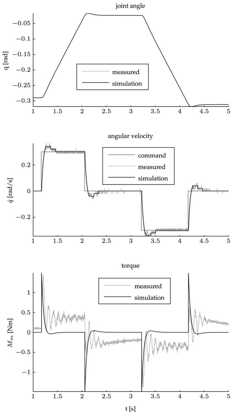
Fig. 5. Simulation results using the identified servo model compared to real measurements (dataset for identification), exemplary for the first shoulder joint (S1)
