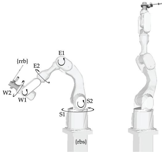
Fig. 7. Differing poses for robot dynamics identification (left) and exemplary verification (right)
