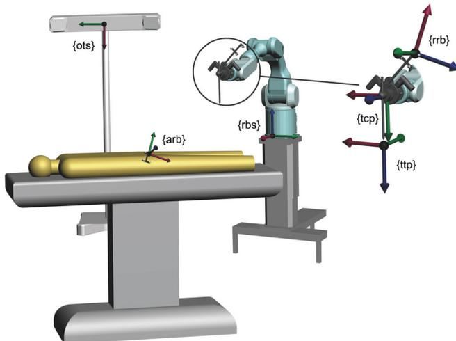
Fig. 2. Coordinate systems -  $\{ots\}$  localizer (optical tracking system),  $\{arb\}$  patient (aim reference body),  $\{rrb\}$  (robot reference body)  $\{rbs\}$  robot base,  $\{tcp\}$  robot wrist (tool center point),  $\{ttp\}$  tool tip
