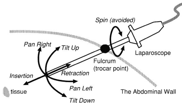
Fig. 4. Movement of endoscope: Since the endoscope is limited due to the insertion site, the endoscope has four degrees of freedom.
