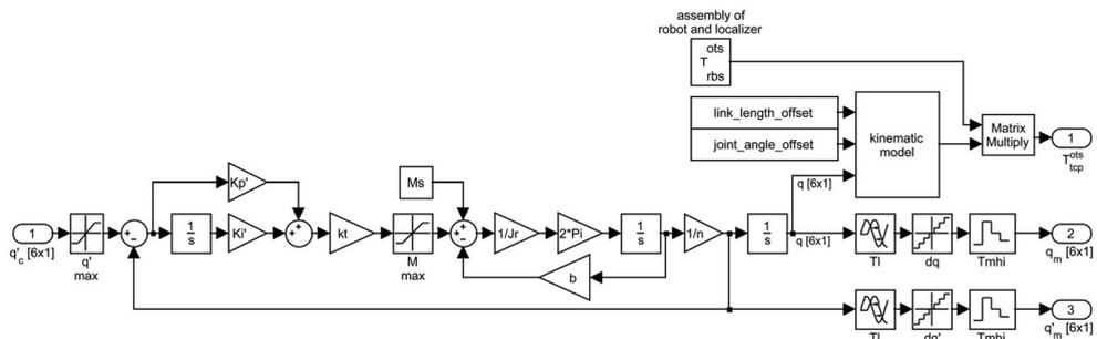
Fig. 4. Robot model - kinematics and joint servo dynamics
