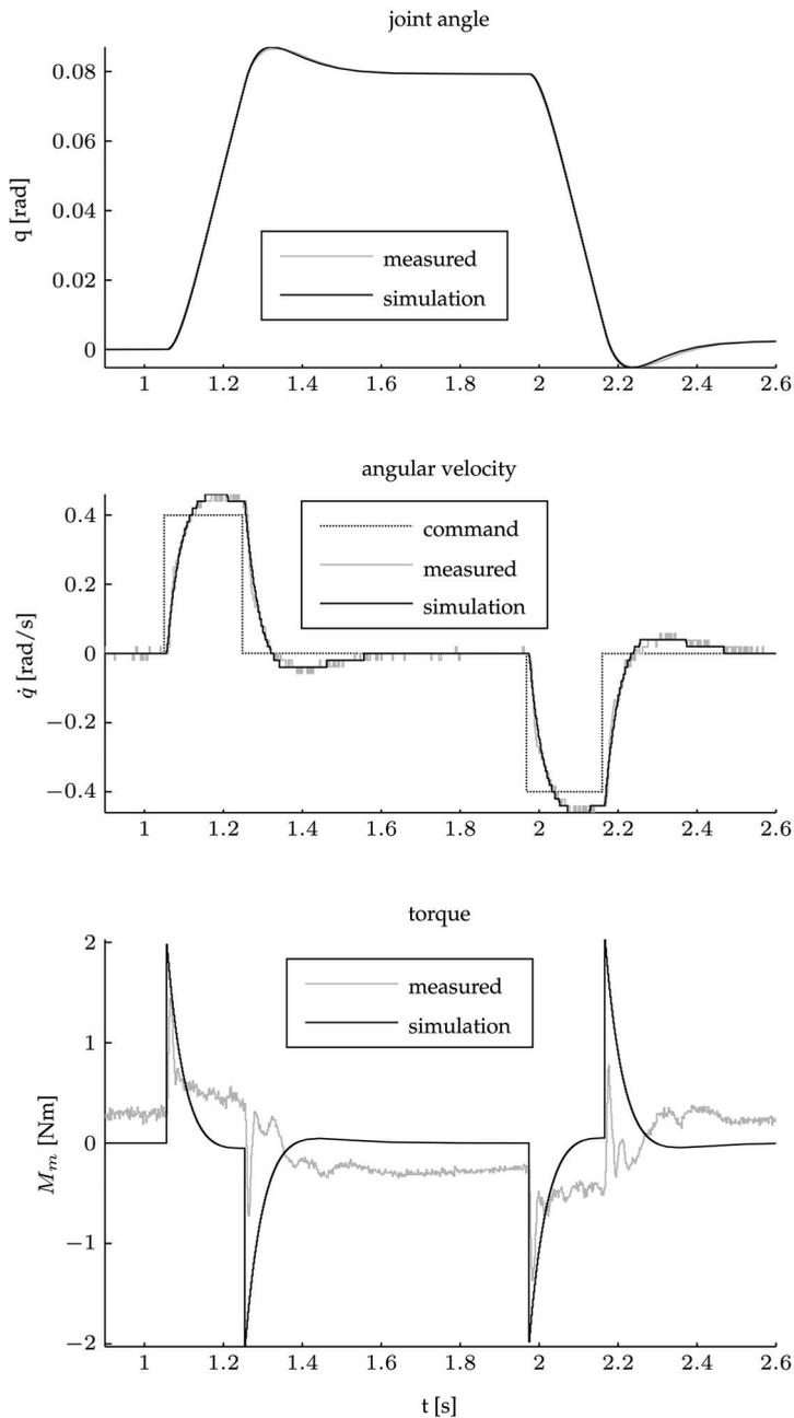
Fig. 6. Simulation results using the identified servo model compared to real measurements for the first shoulder joint (S1) in one exemplary scenario different to the identification scenario
