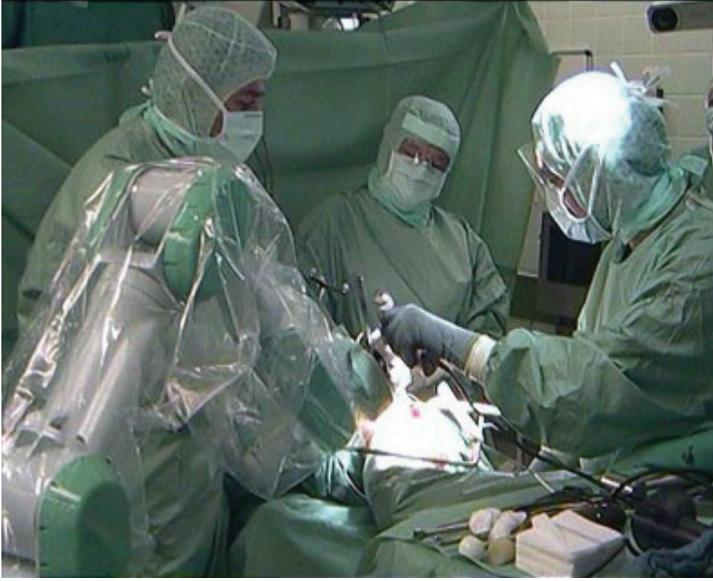
Fig. 1. Clinical trial utilizing the MODICAS assistance robot for total hip arthroplasty implantation
