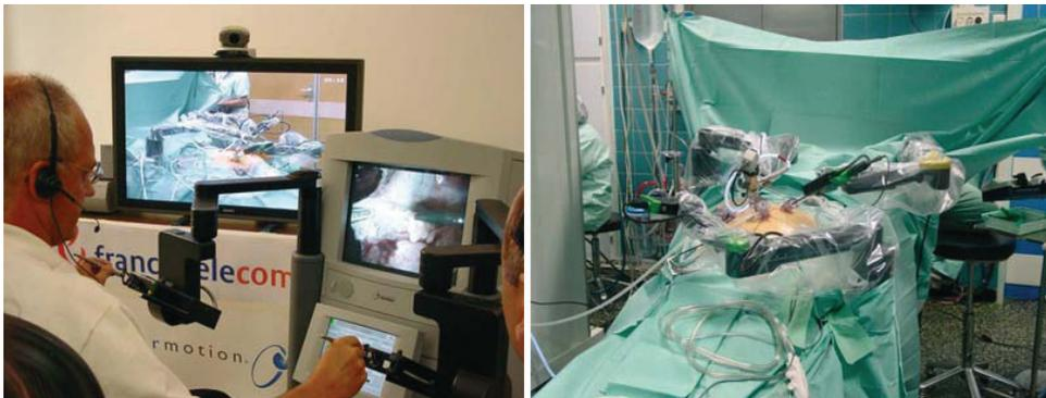
Fig. 4. The Zeus robot during the first intercontinental surgery, the colectomy was performed on the patient in Strasbourg from New York. (Photo: IRCAD)
