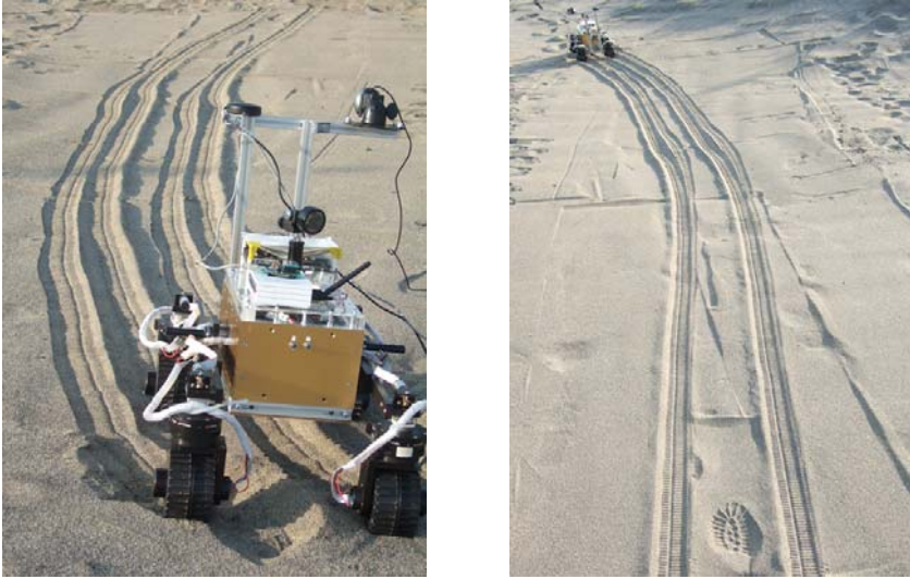
Fig. 11. Position of the rover and wheel traces at the end of the traverse of a sandy slope: a) Front view, b) rear view
