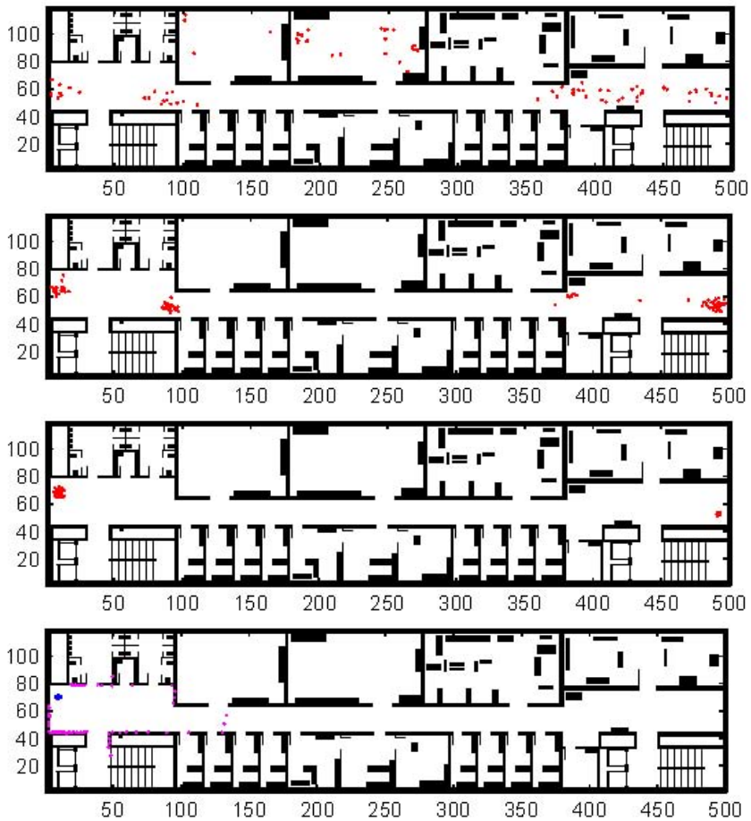
Fig. 10. Convergence process for the worst case pose ( 100, 200, 300, 360 ) of the first perception cycle.
