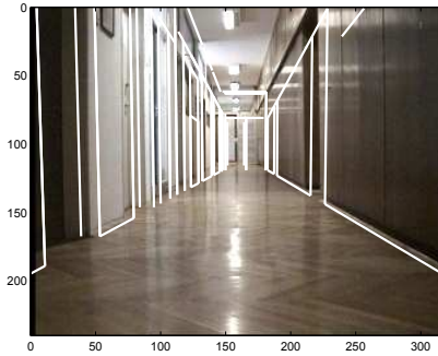
Fig. 19. Superposition of camera view and rendered model before correction
