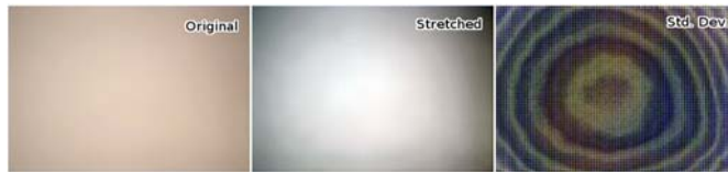
Fig. 6. Radial intensity shift, this noise often occurs on glossy surfaces
