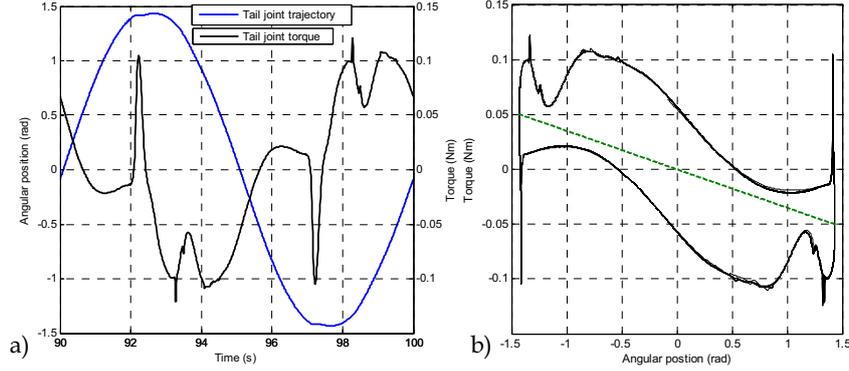
Figure 8. a) Joint position and torque vs. time, b) Joint torque vs. joint position and fitted line
