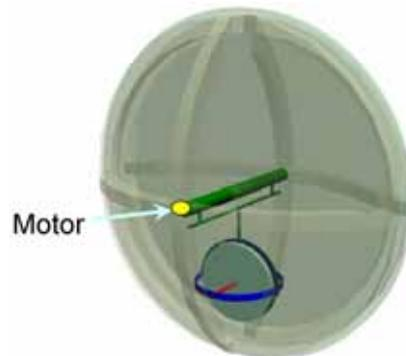
Figure 1. The Basic Design for the Gyroscopic Wheel
