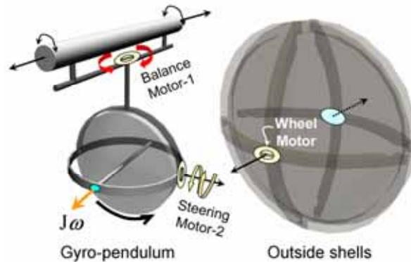
Figure 2. The Graphical Model for the Robot
