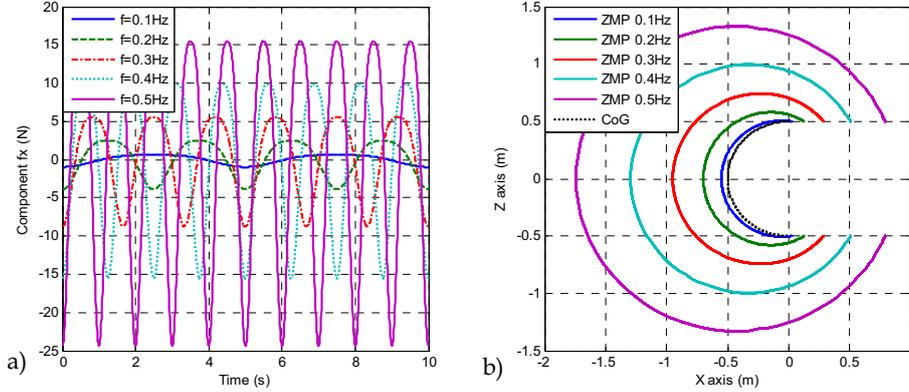
Figure 7. a)  $f_x$  component and b) ZMP and CoG for frequencies between 0,1Hz and 0,5Hz
