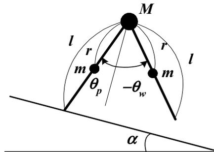
Figure 2. A compass like biped walking robot model
