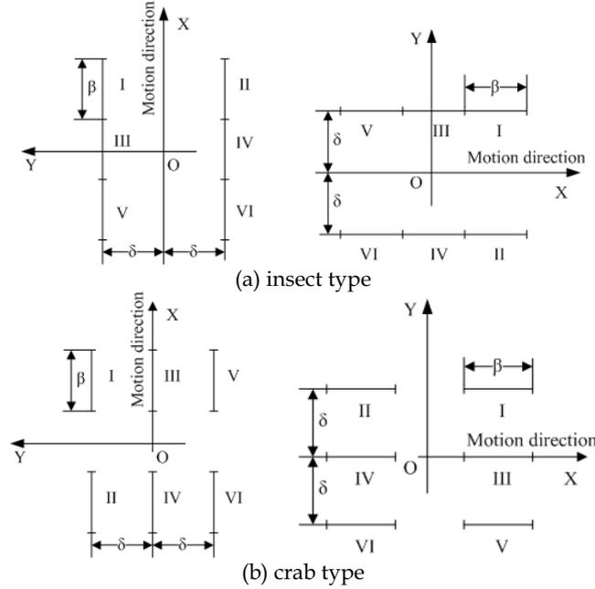
Figure 14. Two typical geometric models in two climbing directions
