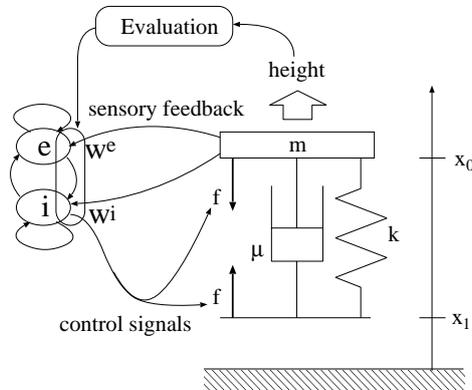
Figure 6. One-dimensional hopping robot. The robot consists of a trunk with mass  $m$  and a leg with a spring component (elastic coefficient:  $k$ ), a damping component (damping coefficient:  $\mu$ ), and a thruster. The oscillator sends control signals to the thruster that generates a force  $f$  between the trunk and the toe and receives the sensory feedback signals from the robot (Nishii, 1999(b))
