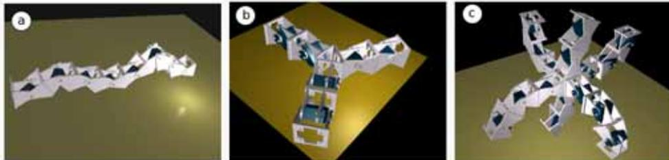
Figure 2. Examples of the three sub-types of chain robots. (a) 1D topology. (b) 2D topology. (c) 3D topology
