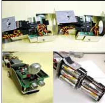
Figure 5. Body, Controller and Power of Snake Robot
