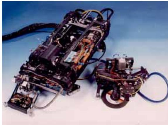
Figure 9. SADIE Robot and Its Tool Packages
