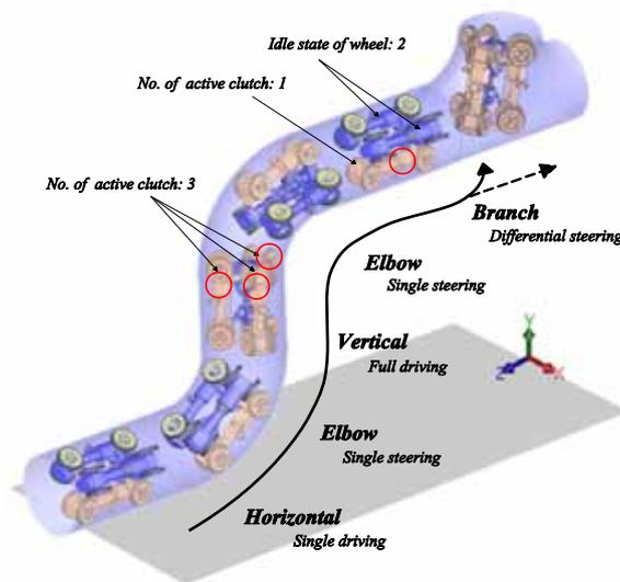
Figure 34. Movement with Selective Driving in Pipelines
