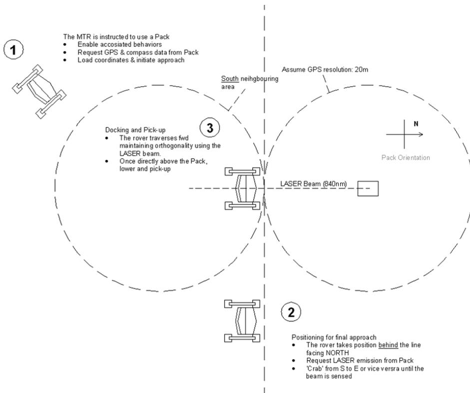
Figure 9. Sequence of events required for the acquisition of a Pack
