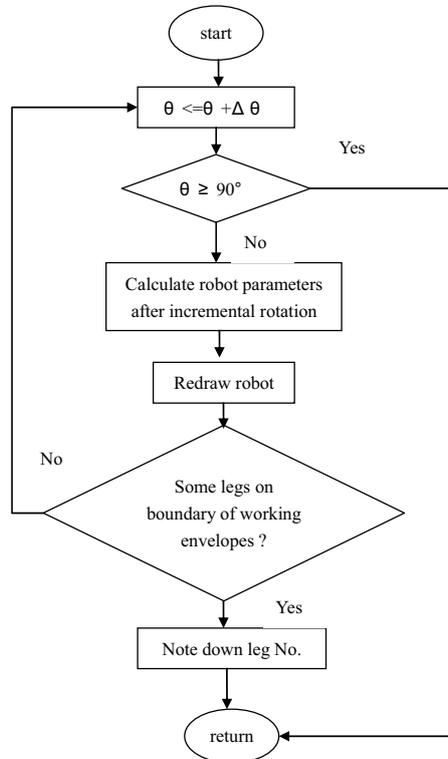
Figure 10. Flowchart of body pitching motion subroutine
