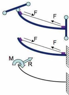
Figure 11. Model for the SMA force analysis. The CGR can be reduced to the study of a cantilever contracted by a SMA wire
