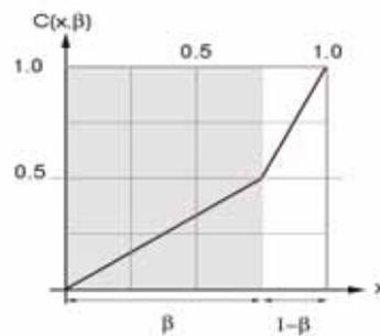
Figure 7. Phase companding curve
