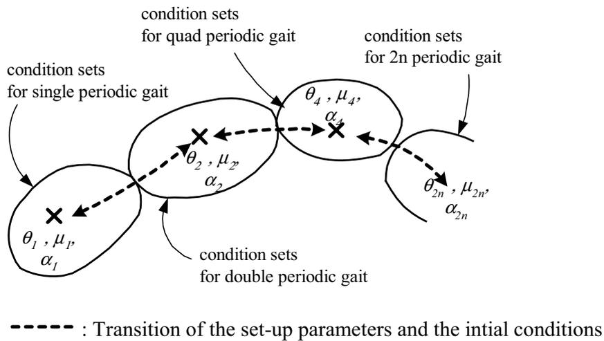
Figure 11. The figure shows that the initial condition sets and the set-up parameters for any kind of the gaits are connected each other and continuously
