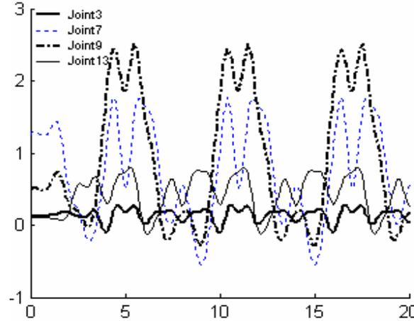
Figure 6. Variation of joint torques ( $\mu=0.3$ ,  $\alpha=\pi/6$ )
