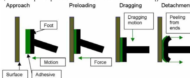
Figure 6. Idealised motion of a compliant robotic foot
