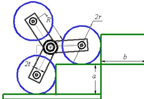
Figure 4. Star-Wheel Parameters
