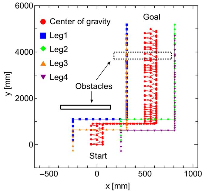
Figure 17. Experimental result of detour and climbing-over action
