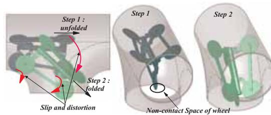
Figure 12. Characteristic features of movement in the branch
