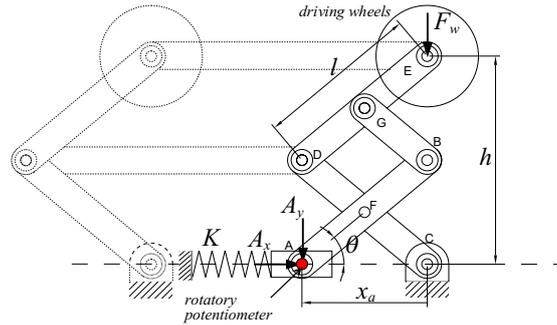
Figure 5. Wheeled leg mechanism of MRINSPECT III
