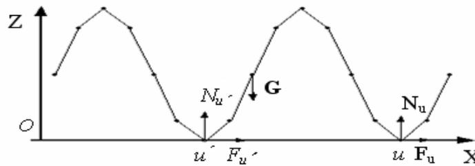
Figure 5. External forces on the snake body
