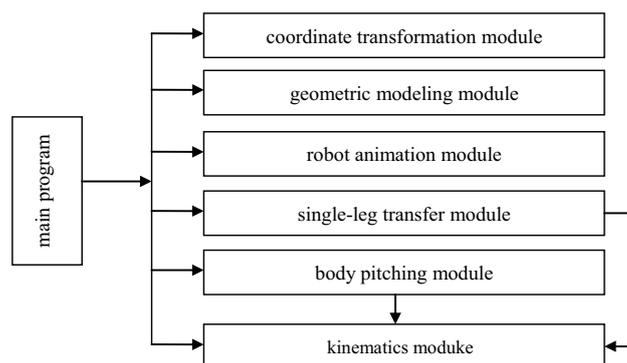
Figure 7. Modular structure of kinematics simulation software
