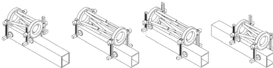
Figure 11. Sequence of the displacements of the robot along a straight trajectory
