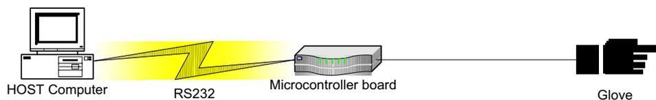
Figure 17. Motion-capturing data glove structure
