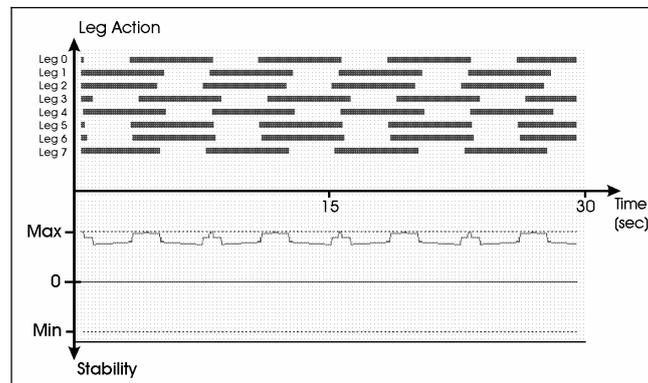
Figure 15. GA-generated walking gait for normal walking on a flat surface
