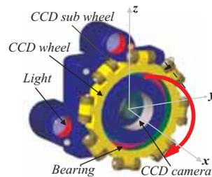
Figure 25. Construction and function of CCD assembly
