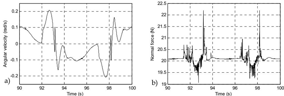
Figure 15. a) Inclination angle velocity and b) normal component of the ground reaction force
