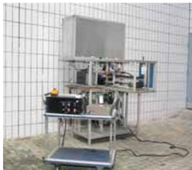
Figure 2. The climbing robot with its ground station and control console
