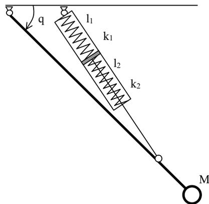
Figure 14. Spring representation of a pneumatic actuator
