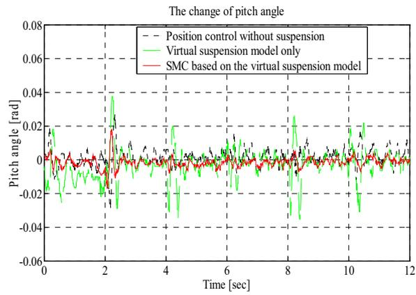
Figure 7. Changes in the direction of pitch angle (Huang, Q. et al, 2007)
