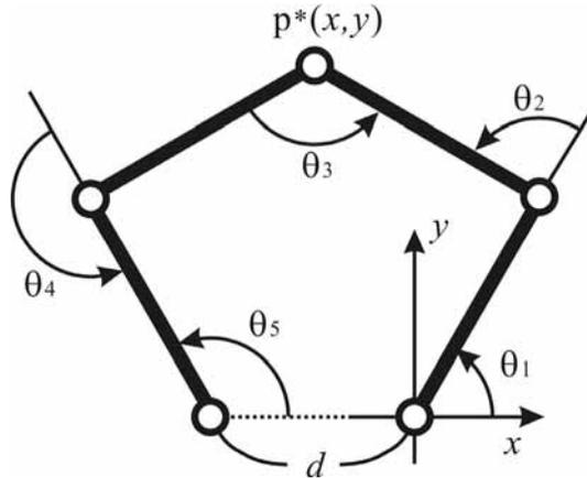
Figure 6. Local coordinate system for inverse kinematics
