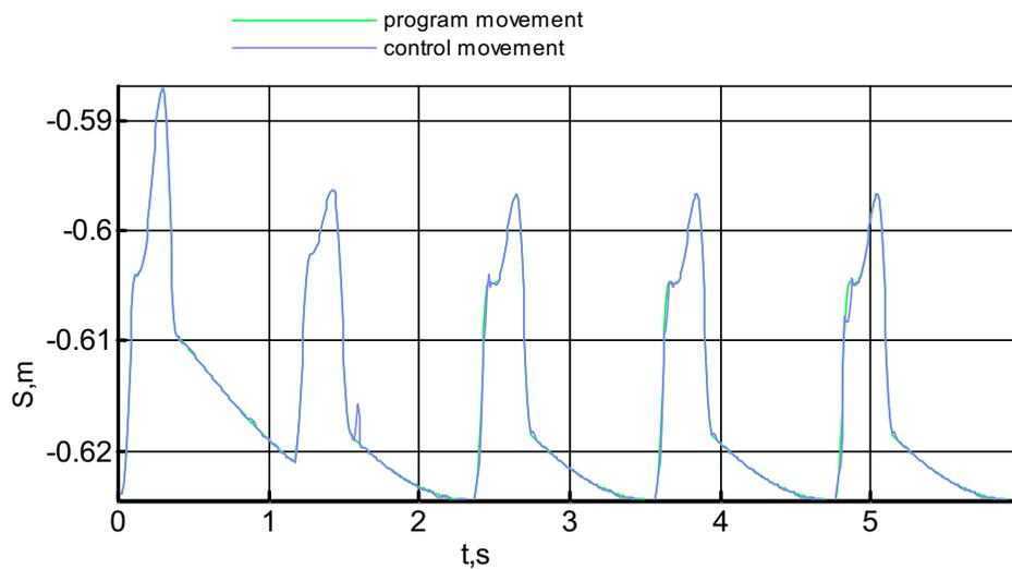
Figure 2. Drive displacement at left front leg, hip – leg actuator
