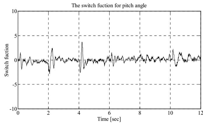
Figure 13. Switching function of SMC based on mode coordinate (Huang, Q. et al, 2007)
