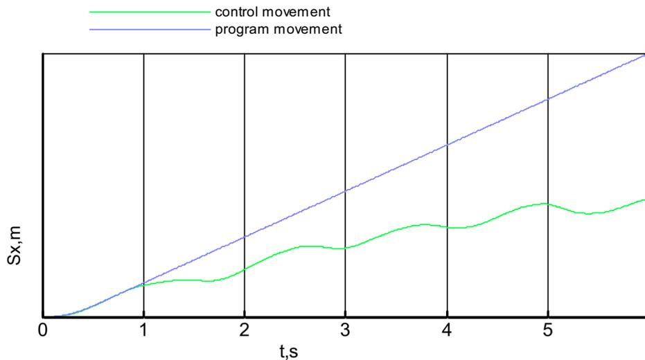
Figure 8. Longitudinal displacement of the cab, control motion is for front shift legs 10 sm
