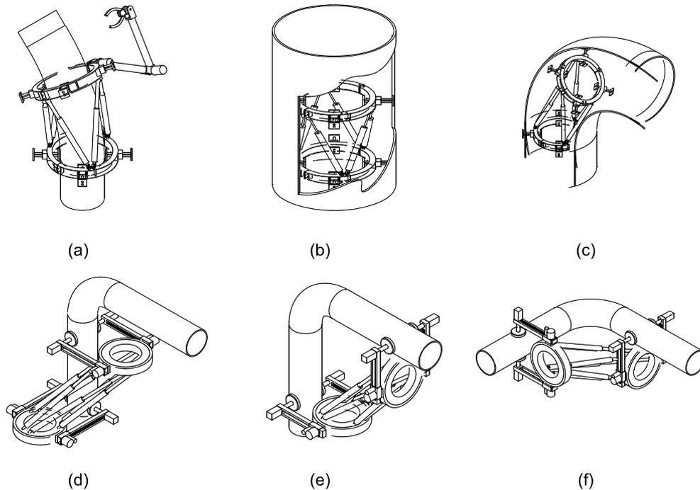
Figure 2. Parallel robots on pipes: (a) robot for working on cables and palm trees, (b), (c) robot for working on curves pipes and tubular structures, (d), (e), (f) some critical configurations of the robot
