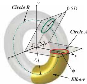
Figure 8. Geometry of the elbow
