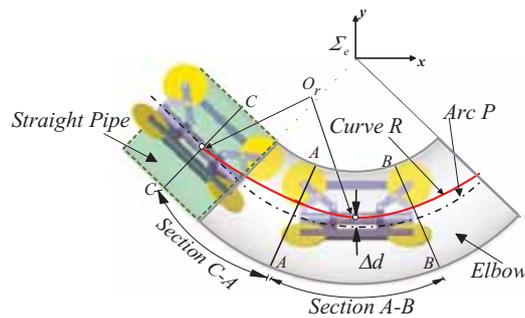
Figure 9. Behavior of the robot entering the elbow
