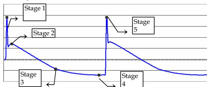
Figure 9. Torque consumption of a Star-Wheel
