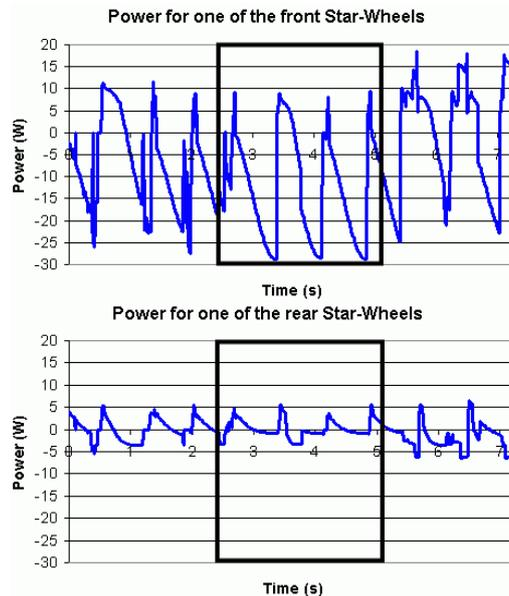
Figure 15. Power consumption for one of the front (Top) and one of the rear (Bottom) Star-Wheels for descending six stairs
