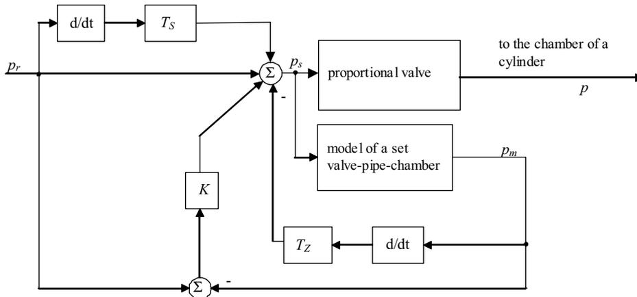
Figure 11. Scheme of a pressure control system
