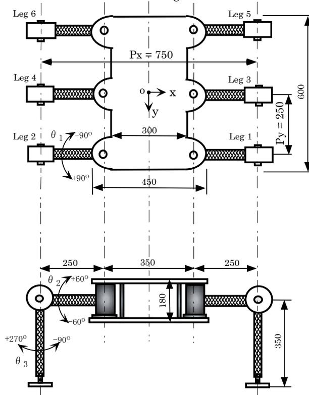
Figure 1. The size of our six-legged walking robot (Huang, Q. et al, 2007)
