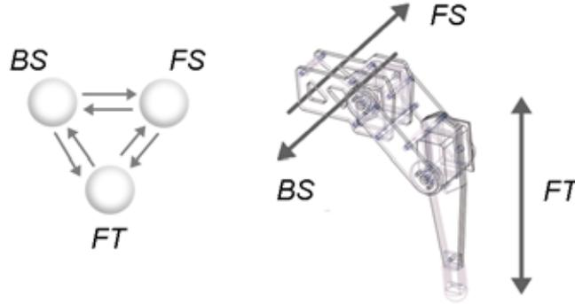
Figure 1. CTRNN based CPG architecture
