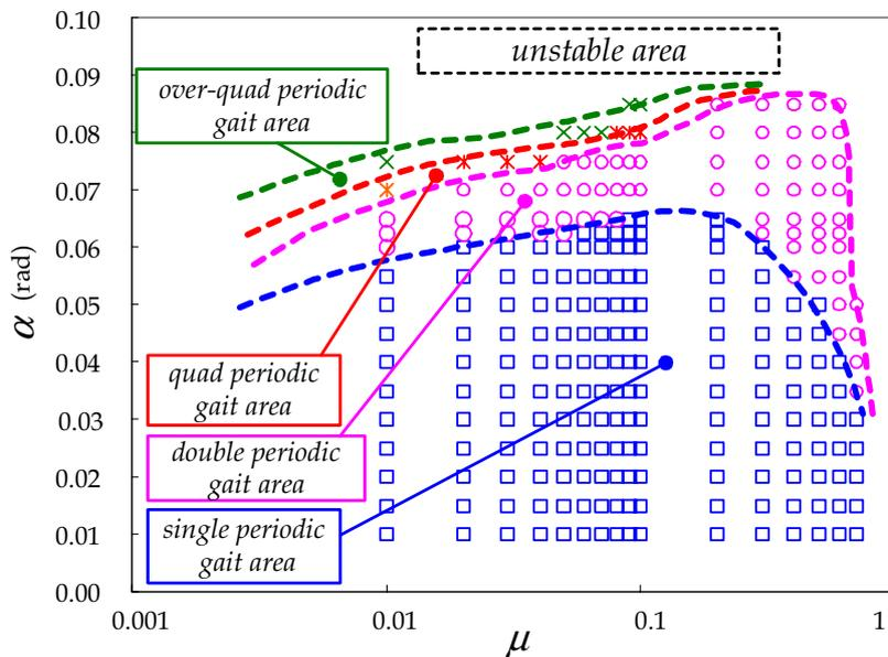
Figure 12. The diagram shows the relation among the parameters  $\alpha$ ,  $\mu$ , and the kind of the gaits. The parameters in the blue square area cause the single periodic gaits; the parameters in the magenta circle area cause the double periodic gaits; the parameters in the red asterisk area causes quad periodic gaits; the parameters in the green cross area causes multi periodic gait; and in the external area the robot can not keep walking
