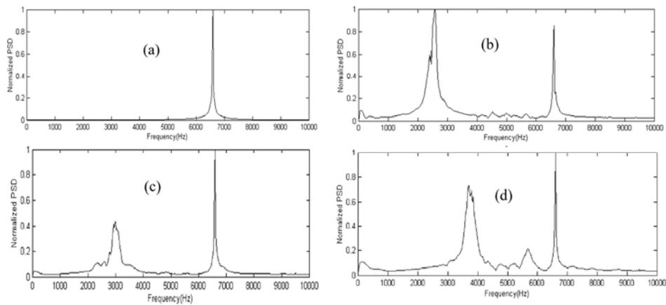
Figure 7. Impact sound feedback spectrum (a) from a solid tile wall, (b) from a tile wall with the debond size 160mm×114mm, (c) with a debond 120mm×114mm, and (d) with a debond 80mm×114mm
