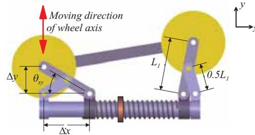
Figure 6. Wheeled leg mechanism of MRINSEPCT IV
