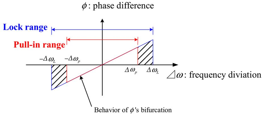
Figure 5. The relation between Pull-in and Lock range and the property of the phase difference
