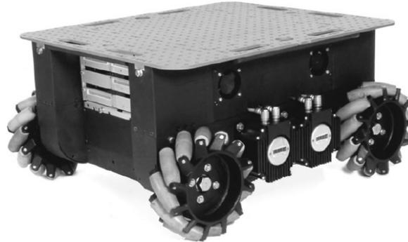
Figure 1. Uranus omnidirectional mobile robot [Muir & Neuman, 1987]
