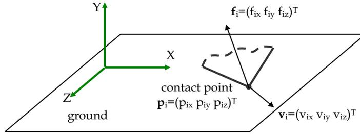
Figure 9. Ground reaction force at a foot contact point  $\mathbf{p}_i$
