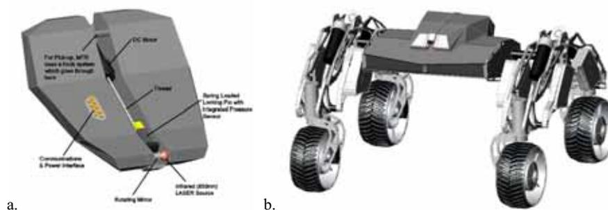
Figure 7. The main elements of the Battery Pack (a), and the MTR equipped with the Pack (b)
