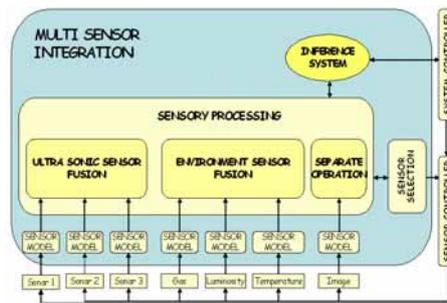
Figure 6. Block Diagram of Sensor Fusion
