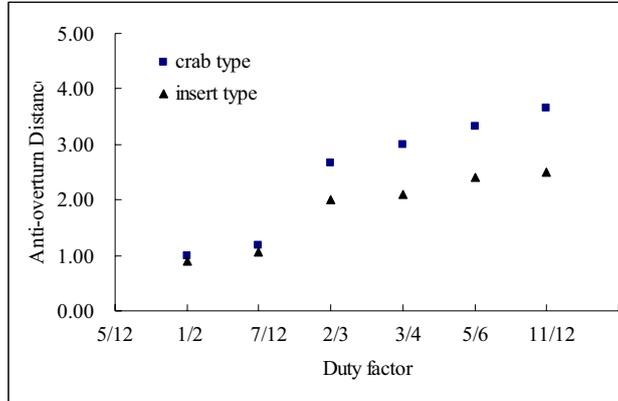
Figure 15. Comparison of AOD with two robot configurations while the wall robot vertically
