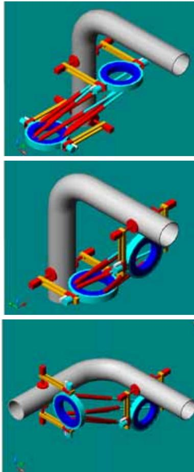
Figure 7. CPR robot climbing outside tubular structures
