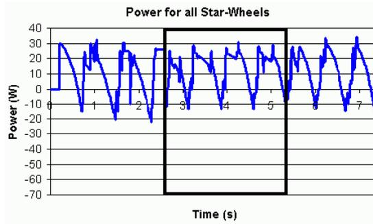
Figure 14. Consumption power for climbing six stairs
