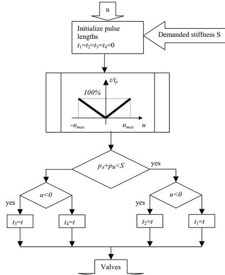
Figure 29. Flow chart for the valve control subsystem
