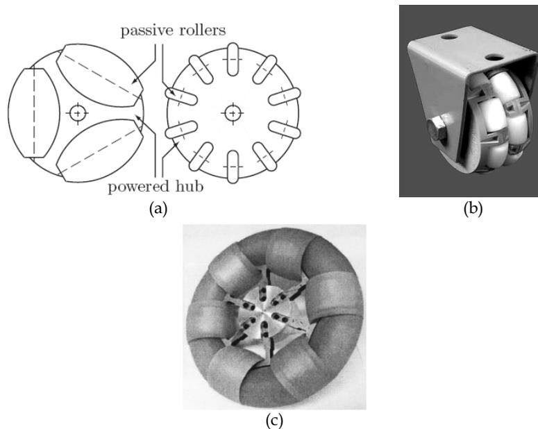
Figure 6. Universal wheel: (a) simple; (b) double; (c) alternate
