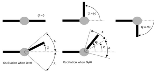
Figure 5. The parameters of the sinusoidal generators
