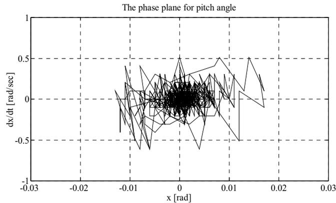
Figure 15. Phase plane of SMC based on mode coordinate (Huang, Q. et al, 2007)
