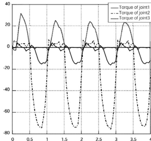
Figure 3. Torques of motors for tripod gait (Huang, Q. et al, 2007)
