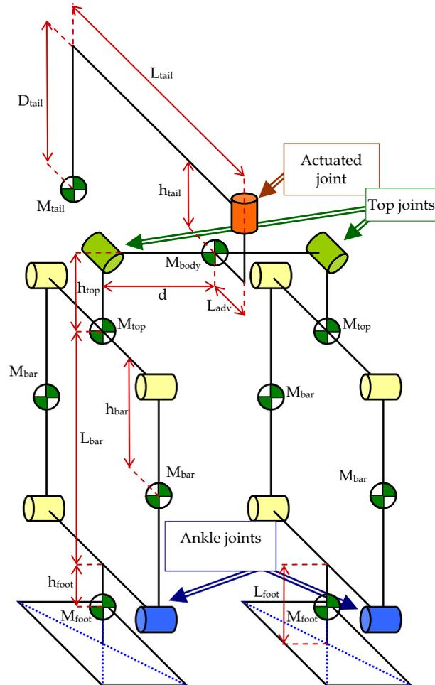
Figure 1. Model of the biped mechanism
