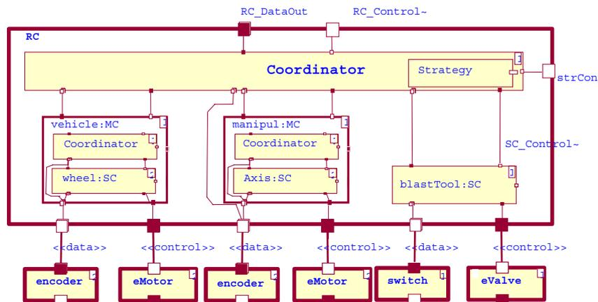
Figure 9. Components of CCAS for Lázaro I control unit
