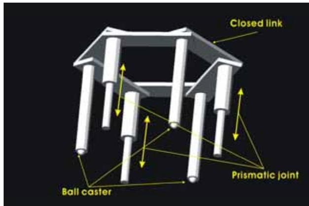
Figure 1. Joint configuration of reduced DOF robot
