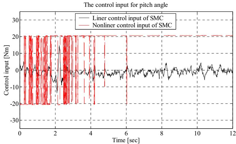
Figure 10. Control input of SMC of servo style (Huang, Q. et al, 2007)
