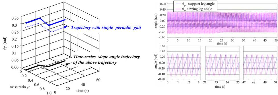
(a) Time-series trajectories of the gait (left) and leg angles (right) when the mass-ratio changes from 0.1 to 0.25 .
