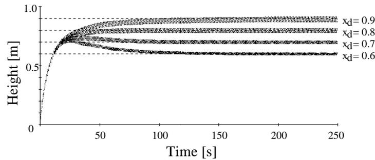
Figure 7. Time profile of the time averaged heights of the trunk of the hopping robot. In this simulation, the evaluation function is set as  $E = x_d - \langle x_0 \rangle$ , where  $x_d = 0.6, 0.7, 0.8, 0.9$  [m] are the desired hopping heights, and  $\langle x_0 \rangle$  is the time averaged height of the trunk (Nishii, 1999(b))
