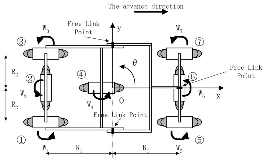
Figure 1. Our holonomic omni-directional vehicle with step-climbing ability
