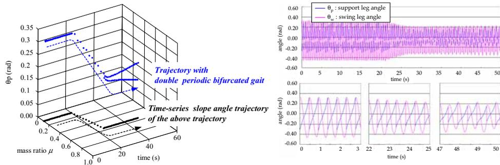
(b) Time-series trajectories of the gait (left) and leg angles (right) when the mass-ratio changes from 0.1 to 0.55 rad.
