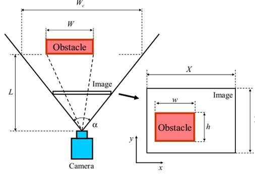
Figure 2. Camera model in top view
