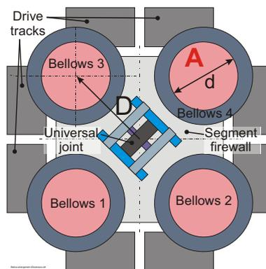
Figure 23. Cross-section of the integrated joint actuator
