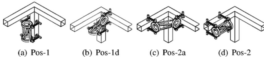
Figure 13. Sequence of postures evading a structural node
