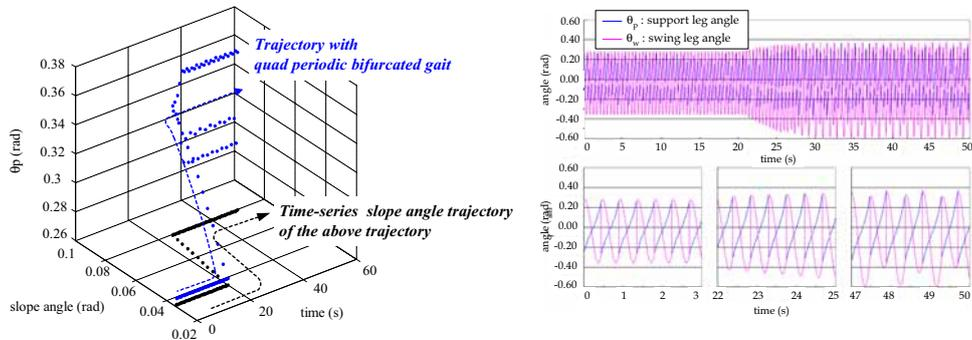
(c) Time-series trajectories of the gait (left) and leg angles (right) when the slope angle changes from 0.035 rad to 0.08 rad.
