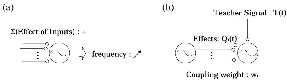
Figure 3. Learning rules for coupled oscillators. (a) The intrinsic frequency  $\omega$  changes according to the sum of the effects of input signals. (b) The coupling weight  $w_i$  changes according to the correlation between the input signal  $Q_i$  and the teacher signal  $T(t)$
