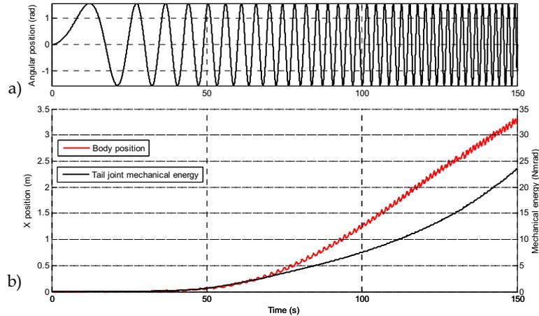
Figure 18. a) Tail joint reference trajectory and, b) body position and energy consumption
