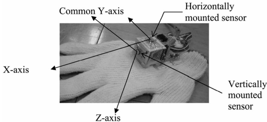
Figure 18. Data glove with two accelerometer sensors mounted on a data glove
