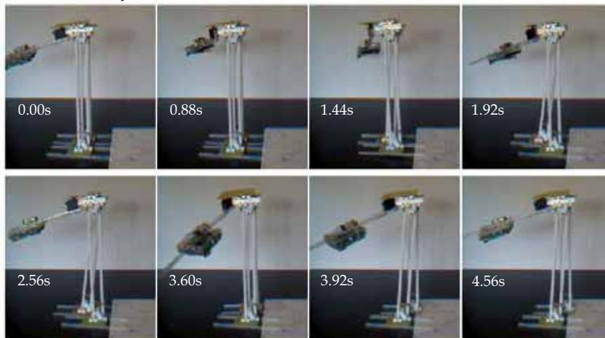
Figure 21. Biped prototype Zappa performing two steps
