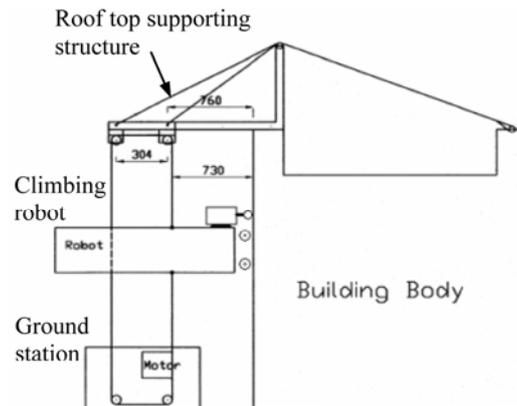
Figure 1. The basic setup of the WIC inspection robot system
