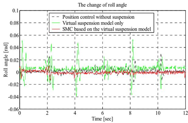
Figure 8. Changes in the direction of roll angle (Huang, Q. et al, 2007)
