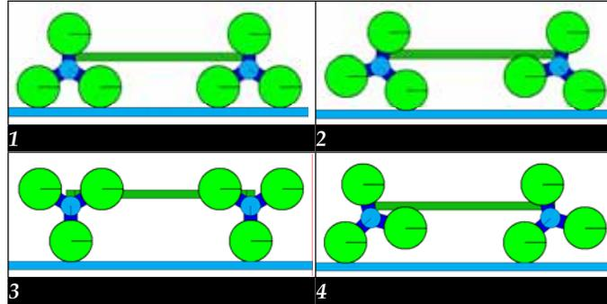
Figure 10. Different stages of Star-Wheels' rotation
