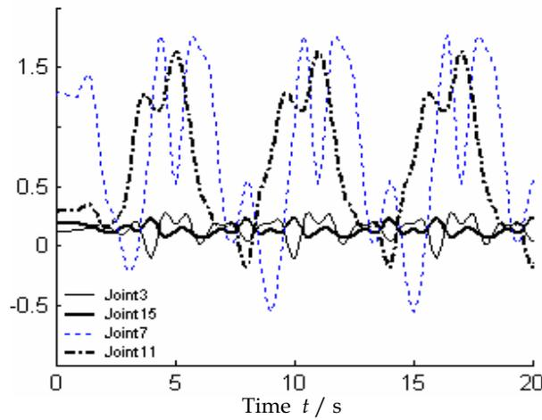
Figure 7. Variation of symmetry joint torque ( $\mu=0.3, \alpha=\pi/6$ )
