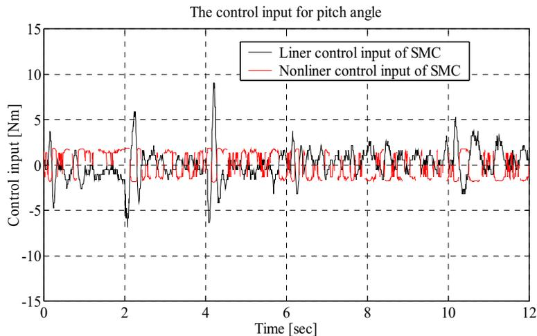
Figure 11. Control input of SMC based on mode coordinate (Huang, Q. et al, 2007)
