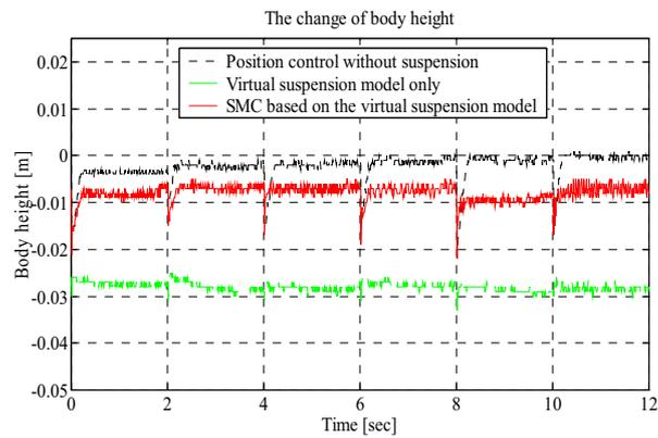
Figure 9. Changes in the vertical direction (Huang, Q. et al, 2007)
