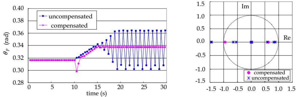
Figure 16. The simulative result of applying the proposed compensation method. The left diagram shows the gait trajectory, and the right diagram shows the absolute maximum of the eigen value of Poincare map ( $|\lambda|_{\max}$ ). As applying the method, the bifurcated gait converges and  $|\lambda|_{\max}$  is less than 1.0
