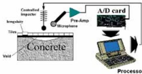
Figure 4. The system block diagram of the impact acoustic inspection device
