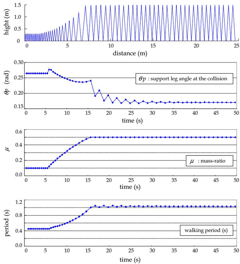
Figure 14. The diagrams show the simulative results of changing the mass-ratio  $\mu$  during the passive dynamic walking
