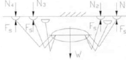
Fig.17. Legged robot climbing on ceilings
