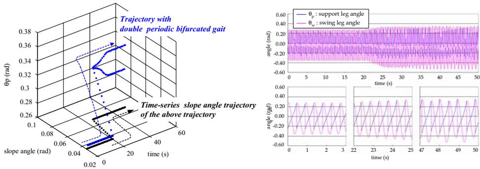
(b) Time-series trajectories of the gait (left) and leg angles (right) when the slope angle changes from 0.035 rad to 0.07 rad.
