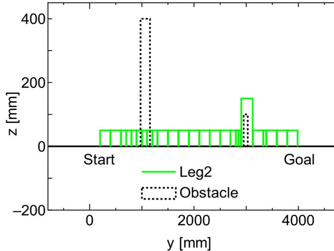
Figure 16. Tip of 2nd leg with a detour and striding action
