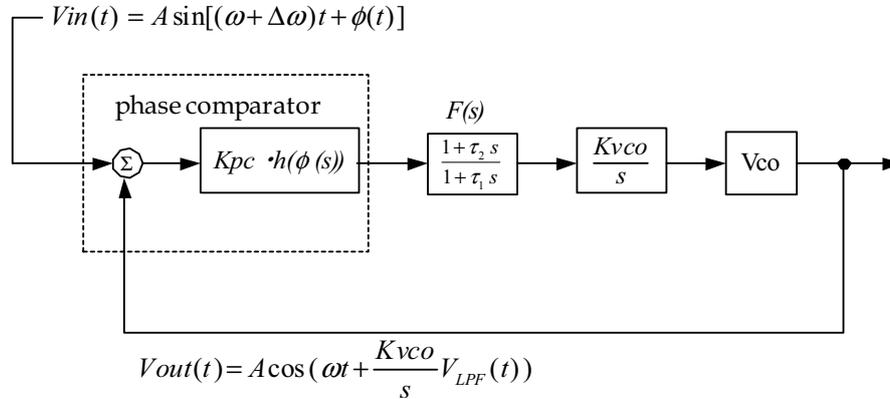
Figure 4. A block diagram of the typical Phase locked loop circuit
