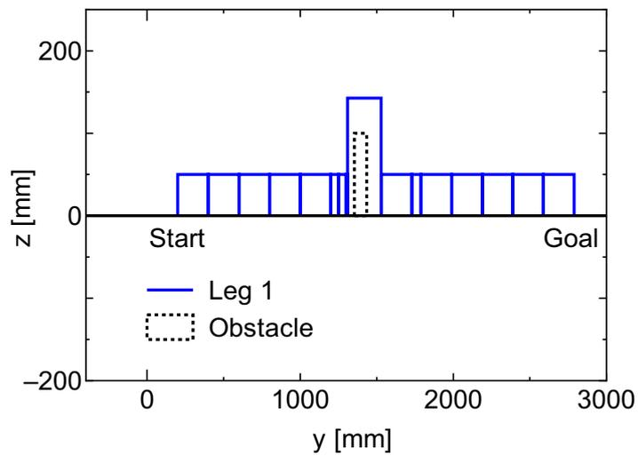
Figure 11. Tip of 1st leg in the experimental result of striding action
