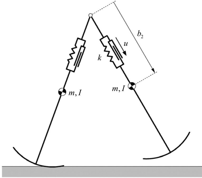
Figure 6. Model of planar telescopic legged biped with elastic elements
