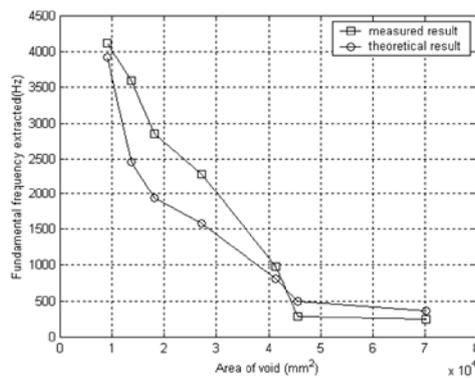
Figure 8. Theoretical and measured fundamental frequency versus debond size
