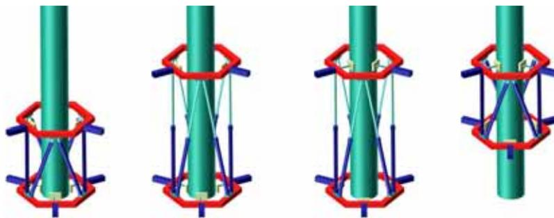
Figure 8. Steps that define the climbing process of a CPR
