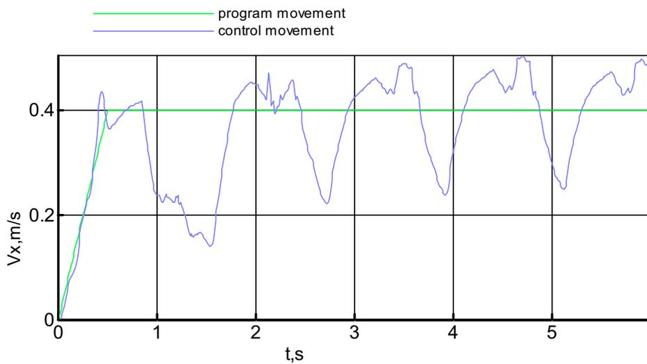
Figure 4. Longitudinal velocity of the cab
