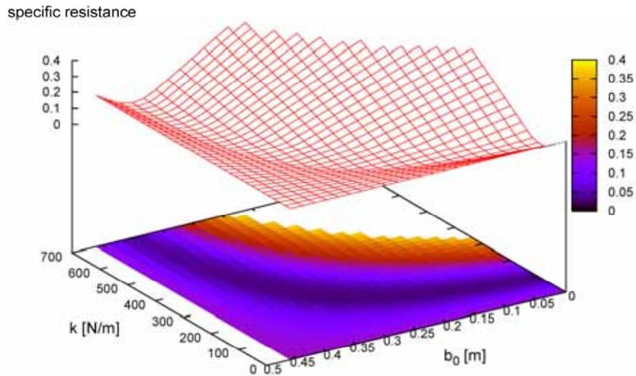
Figure 7. Specific resistance with respect to elastic coefficient and nominal leg length
