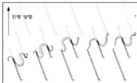
Figure 3. Side-Winding Motion
