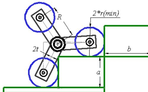
Figure 5. Star-wheel with  $r_{\min}$
