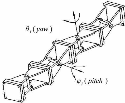
Figure 11. Control model of the two-DOF joints
