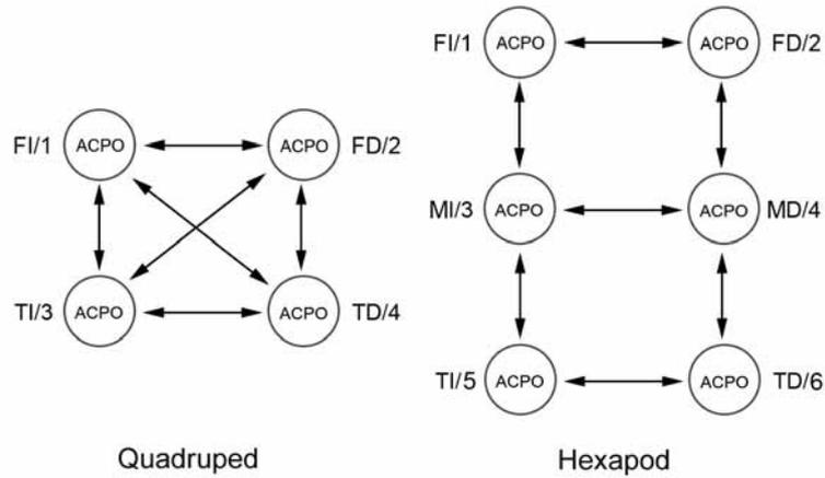
Figure 12. Interconnections schemes for quadruped and hexapod
