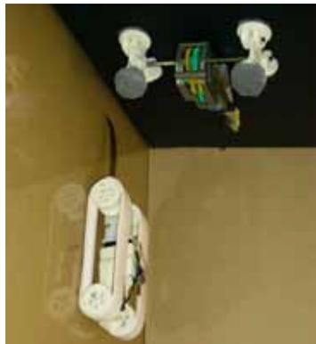
Figure 5. Tank (bottom) and Tri-Leg (top) robots
