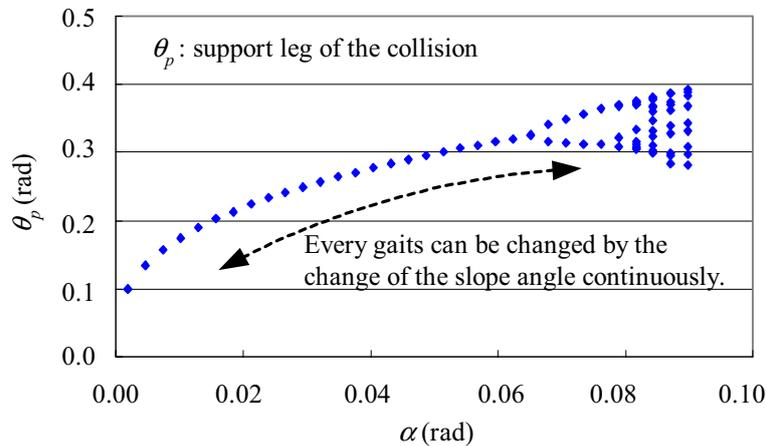
Figure 7. The relation between the slope angle and the gait
