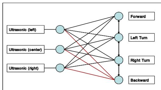
Figure 7. Neural Network using Ultrasonic Sensor Fusion
