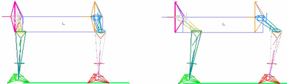
Figure 5. Initial position of the machine, zero shift middle legs position (left), front shift middle legs position 20 sm (right)
