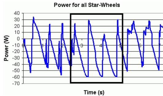
Figure 16. Consumption power for descending six stairs
