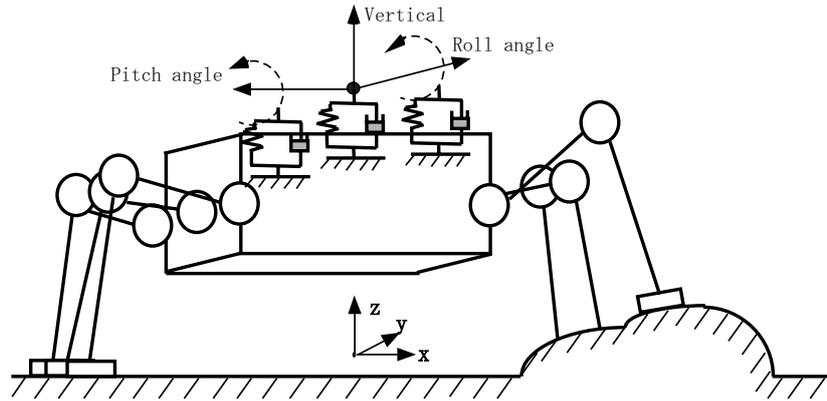
Figure 5. The virtual suspension dynamic model (Huang, Q. et al, 2007)
