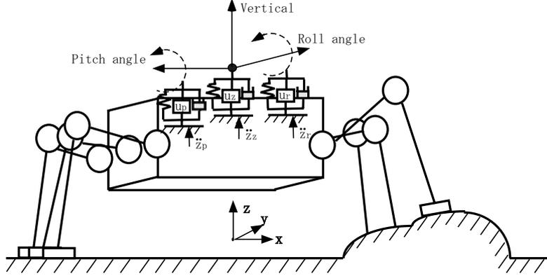
Figure 6. The virtual suspension model considering of active control input and disturbances (Huang, Q. et al, 2007)
