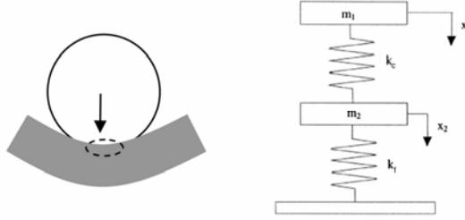
Figure 6. The spring-mass model of impact
