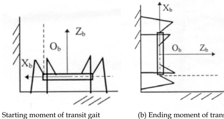
Figure 2. Transit gait of robot from ground to wall
