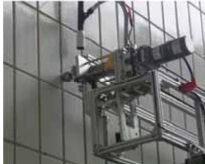
Figure 5. A close-up view of the inspection system in operation
