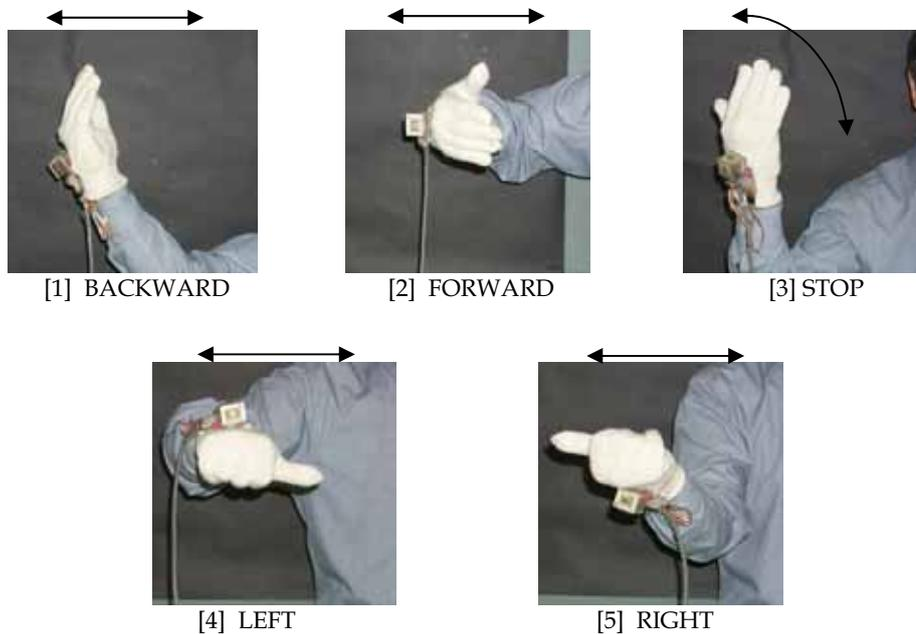
Figure 19. Five prototype gestures with indications of swinging directions
