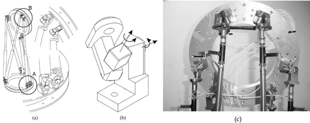
Figure 4. To accomplish postures of  $90^\circ$  between both rings of the robot, it is necessary to modify the spherical and universal joints. (a) Details A and B indicate the necessity of open spherical and universal joints to achieve the orientations between the rings. (b) Modified joints are shown. (c) Upper ring is at  $90^\circ$  with respect to the lower ring, using the modified universal joints
