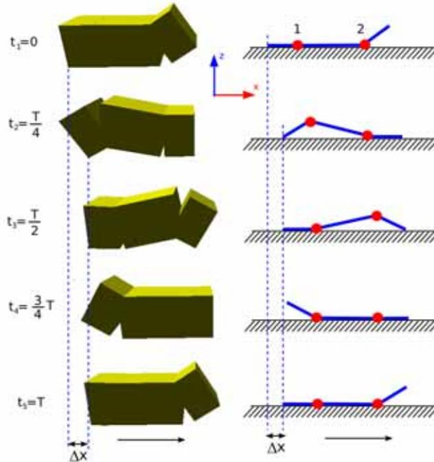
Figure 14. Locomotion of the pitch-pitch (PP) minimal configuration
