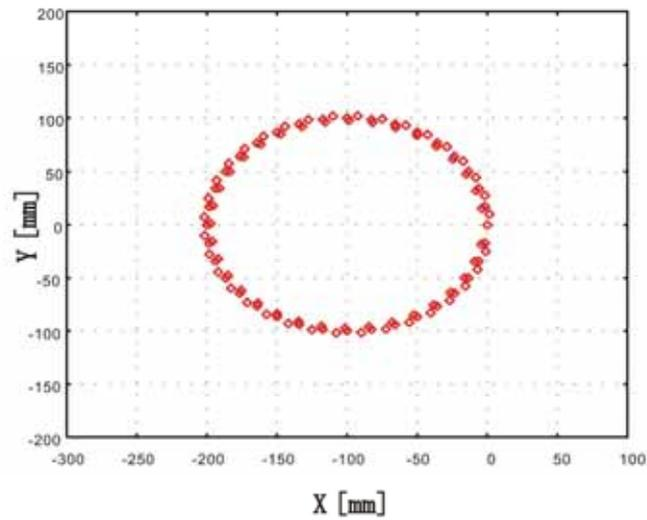
Figure 8. Result of CPB in circular walk
