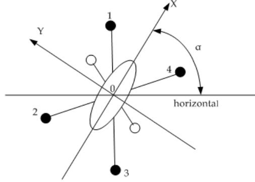
Figure 12. Legged wall robot side view with body frame attached (\* Black circle denoted the suckers in support status)
