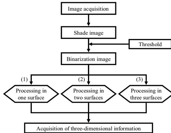
Figure 5. Flow of image data processing
