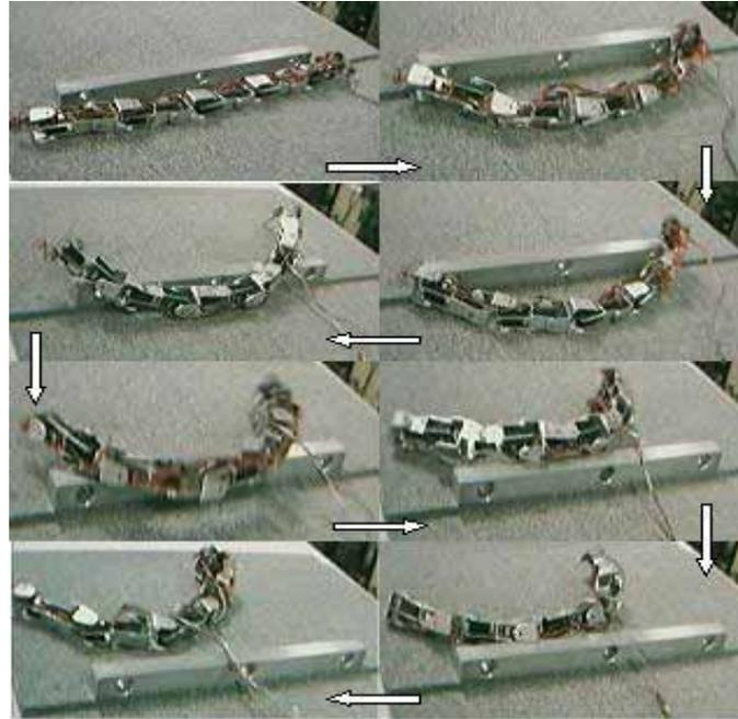
Figure 13. Rolling over an obstacle of the snake robot
