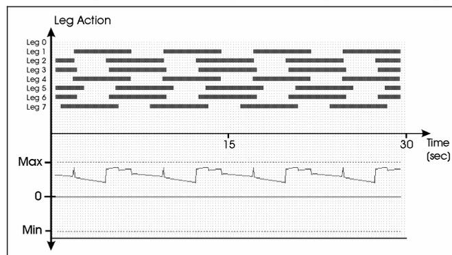
Figure 16. GA-generated walking gait for when one leg is made inoperative
