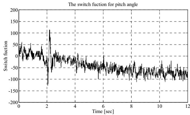
Figure 12. Switching function of SMC of servo style (Huang, Q. et al, 2007)
