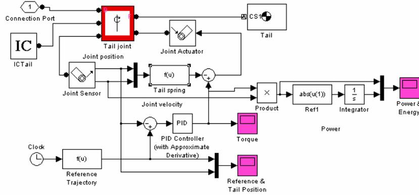
Figure 11. Blocks and signals into the Tail subsystem
