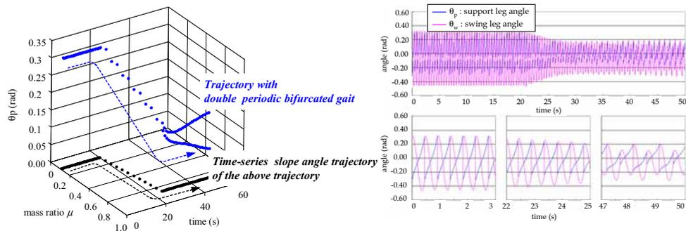
(c) Time-series trajectories of the gait (left) and leg angles (right) when the mass-ratio changes from 0.1 rad to 0.65.
