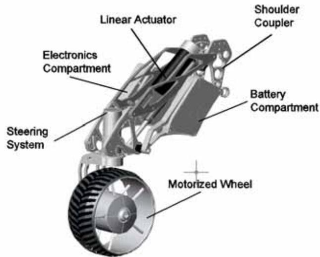
Figure 3. A CAD illustration, showing the main elements of a leg
