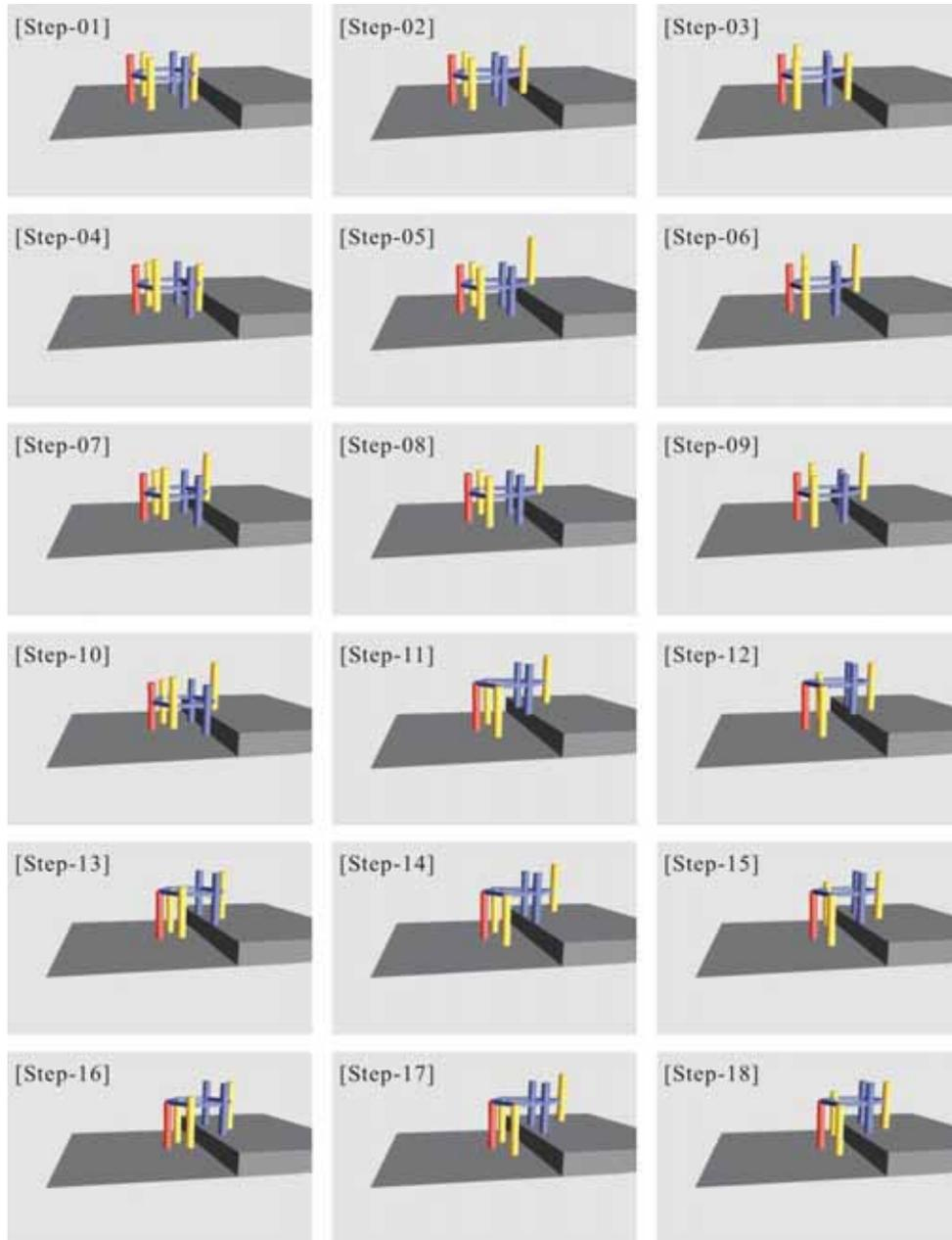
Figure 10(a). Sequence for walk over a step (from Step 1 to 18)
