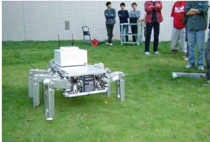
Figure 4. The developed six-legged walking robot (Huang, Q. et al, 2007)
