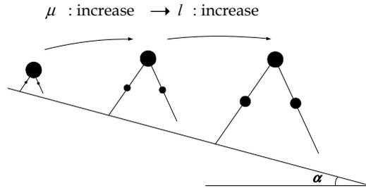
Figure 13. The figure shows that the leg length becomes long as increasing the mass-ratio  $\mu$ . Suppose the mass density of the leg is constant, the changes of the mass (or the mass-ratio) cause the changes of the leg length of the robot in proportion to the rate of the mass (or the mass-ratio) change
