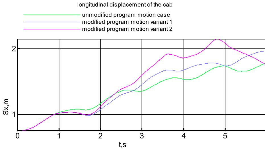
Figure 9. Longitudinal displacement of the cab for control motion for front legs shift 10 sm
