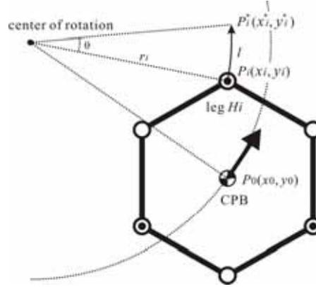
Figure 5. Coordinate system for rotational walk
