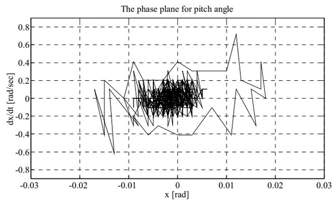
Figure 14. Phase plane of SMC of servo style (Huang, Q. et al, 2007)
