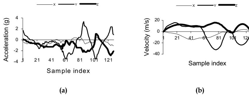
Figure 20. Recorded acceleration and generated velocity profiles of a typical STOP gesture
