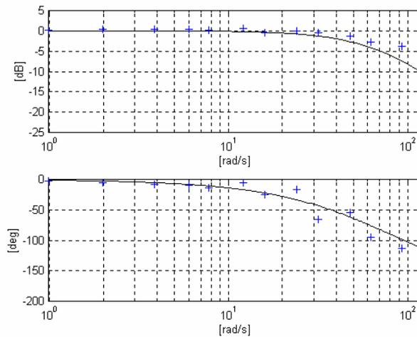
Figure 9. Bode plots of a pneumatic drive: proportional valve mounted directly to the cylinder and volume of a chamber 41cm<sup>3</sup>
