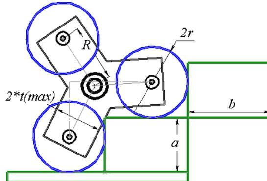
Figure 7. Star-wheel under  $t_{\max}$  condition
