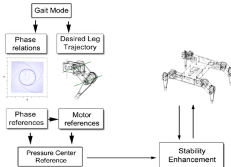
Figure 11. System architecture. CPG model with force feedback
