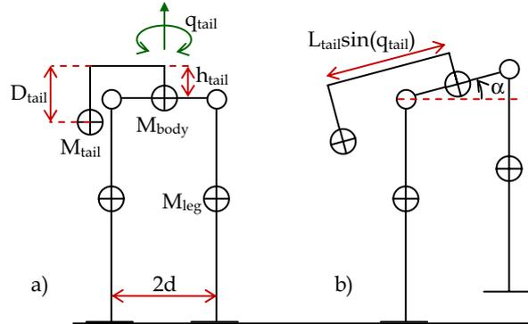
Figure 3. a) Double support configuration, b) Configuration with a raised foot
