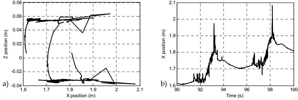
Figure 16. a) ZMP displacement and b) X component of the ZMP during one stride
