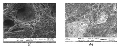
Fig.13. (a and b) - Microstructure of formulation 2 sintered in conventional oven at temperatures of 1500  $^{\circ}$ C (a) and 1550  $^{\circ}$ C (b)
