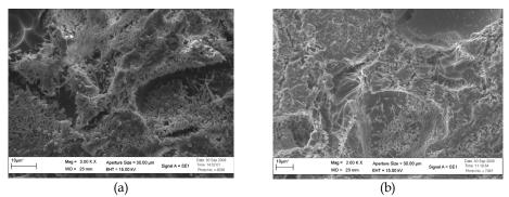
Fig. 12. (a and b) - Microstructure of formulation 1 sintered in conventional oven at temperatures of 1500  $^{\circ}$ C (a) and 1550  $^{\circ}$ C (b)
