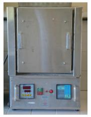
Fig. 3. Conventional oven used in the burning of the specimens
