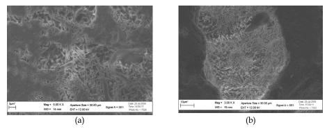
Fig. 14. (a and b) - Microstructure of formulation 3 sintered in conventional oven at temperatures of 1500  $^{\circ}$ C (a) and 1550  $^{\circ}$ C (b)
