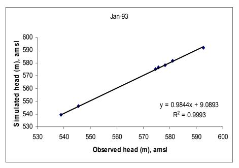
Fig. 9. Observed and simulated groundwater levels during calibration
