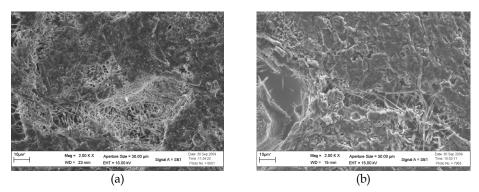
Fig. 15. (a and b) - Microstructure of formulation 4 sintered in conventional oven at temperatures of 1500  $^{\circ}$ C (a) and 1550  $^{\circ}$ C (b)
