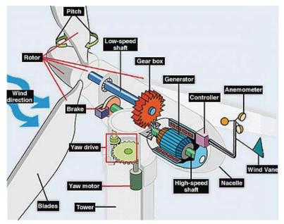
Fig. 1. Wind turbine parts
