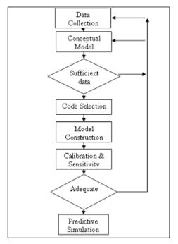
Fig. 3. Groundwater flow methodology (ASTM, D5447-2004)
