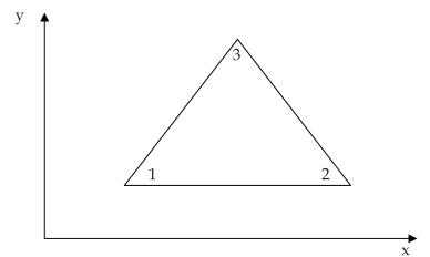
Fig. 4. Linear triangular finite element
