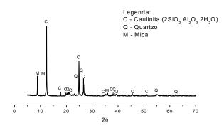
Fig. 5. XRD of the residue of kaolin
