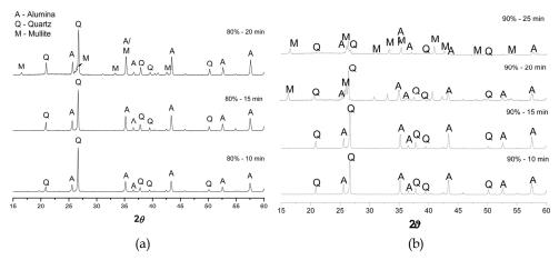
Fig. 18. (a and b) – XRD patterns of formulation 2 sintered in microwave at 80% power (a) (in times of 10, 15 and 20 minutes) and the power of 90% (b) (in times of 10, 15, 20 and 25 minutes)
