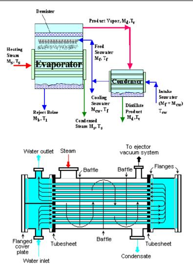
Fig. 7. Desalination process and heat exchanger (condenser)
