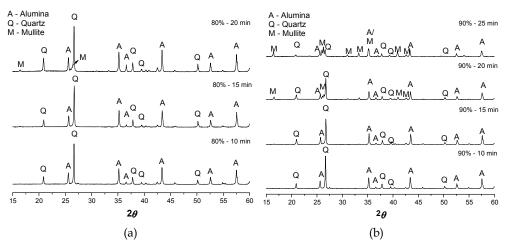
Fig. 21. (a and b) – XRD patterns of formulation 5 sintered in microwave at 80% power (a) (in times of 10, 15 and 20 minutes) and the power of 90% (b) (in times of 10, 15, 20 and 25 minutes)
