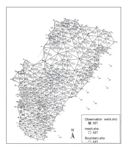
Fig. 8. Finite element mesh for Varada river basin (mod. after Ramesh & Mahesha, 2008)
