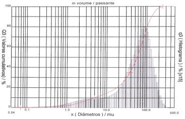
Fig. 6. Particle size distribution of the residual kaolin
