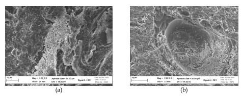
Fig. 16. (a and b) - Microstructure of formulation 5 sintered in conventional oven at temperatures of 1500  $^{\circ}$ C (a) and 1550  $^{\circ}$ C (b)
