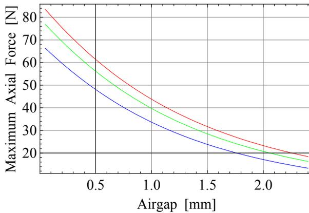
Fig. 11. Maximum axial force versus the air gap radial dimension for several ring radial thicknesses.  $h = 3\text{mm}$ . Blue:  $r_1 = 25\text{mm}, r_2 = 28\text{mm}, r_3 = 21\text{mm}, r_4 = 24\text{mm}$  Radial thickness  $r_2 - r_1 = r_4 - r_3 = 3\text{mm}$ , Green: Radial thickness  $4\text{mm}$ , Red: Radial thickness  $5\text{mm}$ .
