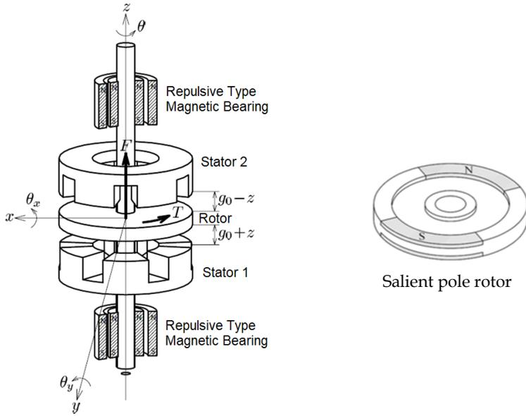
Fig. 4. Detail structure and coordinates of the AGBM
