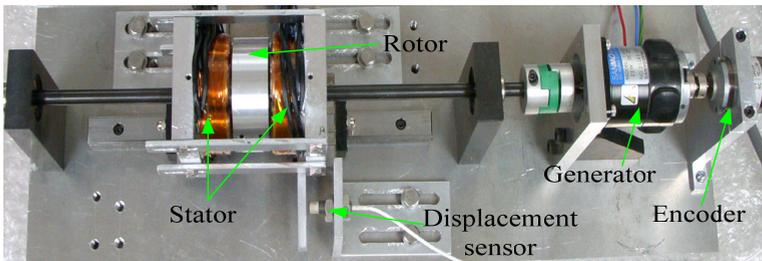
Fig. 14. Picture of the experimental setup
