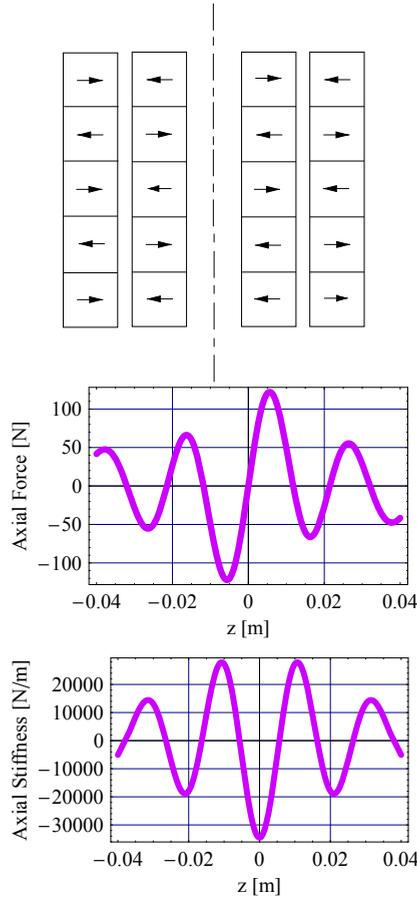
Fig. 28. Axial force and stiffness versus axial displacement for a stack of five ring permanent magnets with radial polarizations;  $r_1 = 0.01$  m,  $r_2 = 0.02$  m,  $r_3 = 0.03$  m,  $r_4 = 0.04$  m,  $J = 1$  T, height of each ring permanent magnet = 0.01 m
