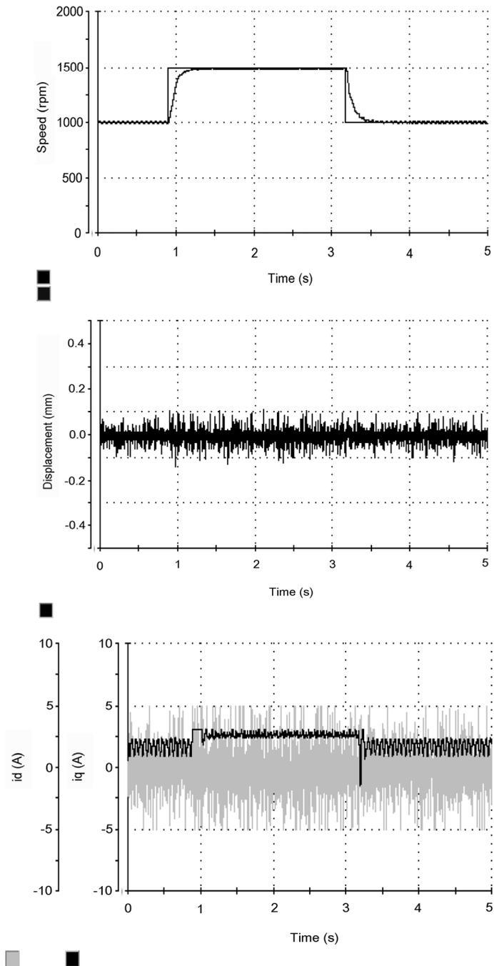
Fig. 21. Currents and displacement when rotor speed was changed
