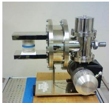
Fig. 7. The bulk twined heads pulse tube cryocooler
