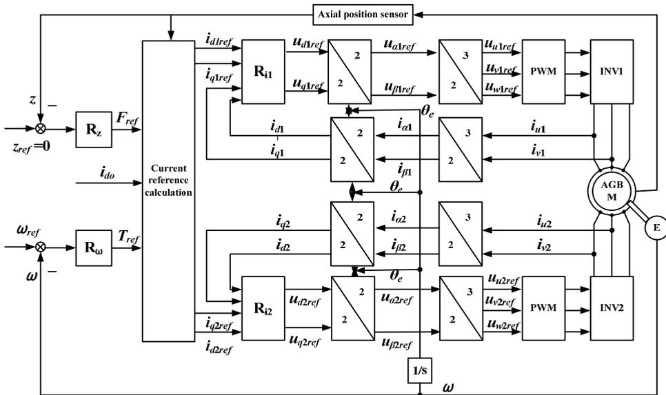
Fig. 10. Control structure for the AGBM.
