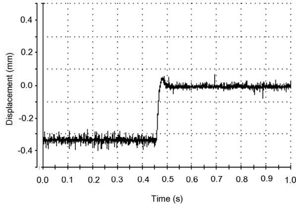
Fig. 17. Response of axial displacement at zero speed
