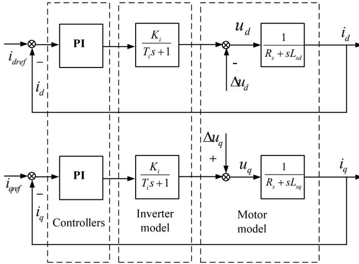
Fig. 11. Decoupled current control loop
