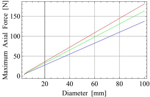
Fig. 10. Maximum axial force versus the air gap perimeter for several ring radial thicknesses. Air gap 1mm,  $h = 3mm$ . Blue:  $r_1 = 25mm, r_2 = 28mm, r_3 = 21mm, r_4 = 24mm$  Radial thickness  $r_2 - r_1 = r_4 - r_3 = 3mm$ , Green: Radial thickness 4mm, Red: Radial thickness 5mm.
