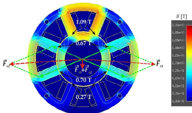
Fig. 6. Magnetic field distribution for the case  $i_x = 0$  A,  $i_y = 3$  A,  $I_0 = 5$  A, and  $x = y = 0$  mm with air gap values of the flux density and vector analysis of a radial force of a pair of electromagnets in the  $x$  axis
