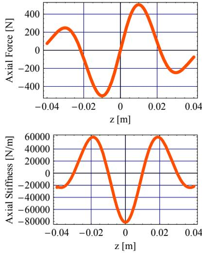
Fig. 27. Axial force and stiffness versus axial displacement for a stack of five ring permanent magnets with perpendicular polarizations;  $r_1 = 0.01$  m,  $r_2 = 0.02$  m,  $r_3 = 0.03$  m,  $r_4 = 0.04$  m,  $J = 1$  T, height of each ring permanent magnet = 0.01 m
