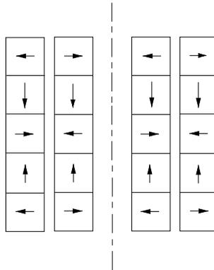
Fig. 26. Cross-section of a stack of five ring permanent magnets with perpendicular polarizations;  $r_1 = 0.01$  m,  $r_2 = 0.02$  m,  $r_3 = 0.03$  m,  $r_4 = 0.04$  m,  $J = 1$  T, height of each ring permanent magnet = 0.01 m
