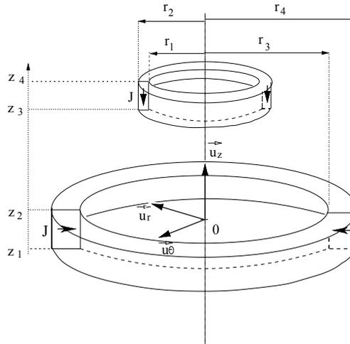
Fig. 24. Ring permanent magnets with perpendicular polarizations.
