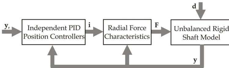
Fig. 15. Structure of the closed-loop AMB system
