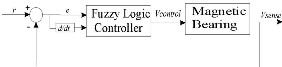
Fig. 7. FLC for MBC500 magnetic bearing system
