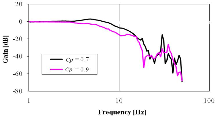
Fig. 14. Transmissibility characteristics of the isolation table.
