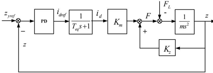
Fig. 12. Axial displacement control loop
