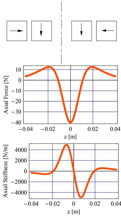
Fig. 25. Axial force axial stiffness versus axial displacement for two ring permanent magnets with perpendicular polarizations;  $r_1 = 0.01$  m,  $r_2 = 0.02$  m,  $r_3 = 0.03$  m,  $r_4 = 0.04$  m,  $z_2 - z_1 = z_4 - z_3 = 0.1$  m,  $J = 1$  T
