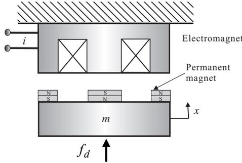
Fig. 2. Model of a zero-power controlled magnetic levitation
