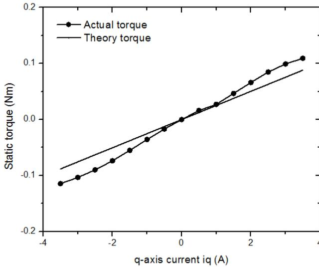
Fig. 9. Relation between rotational torque and q-axis current
