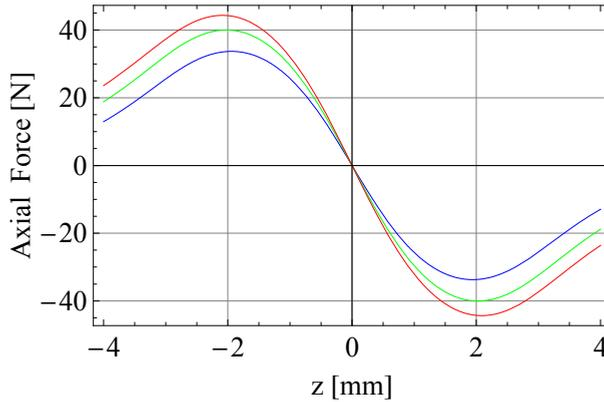
Fig. 8. Axial force for several radial thicknesses. Blue:  $r_1 = 25\text{mm}, r_2 = 28\text{mm}, r_3 = 21\text{mm}, r_4 = 24\text{mm}, h = 3\text{mm}$ , air gap  $1\text{mm}$ , Radial thickness  $r_2 - r_1 = r_4 - r_3 = 3\text{mm}$ , Green:  $4\text{mm}$ , Red:  $5\text{mm}$ .
