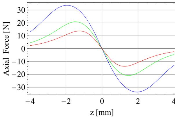
Fig. 5. Axial force for ring small heights. Blue:  $r_1 = 25\text{mm}, r_2 = 28\text{mm}, r_3 = 21\text{mm}, r_4 = 24\text{mm}$ , air gap  $1\text{mm}$   $h = 3\text{mm}$ , Green:  $h = 2\text{mm}$ , Red:  $h = 1.5\text{mm}$ .
