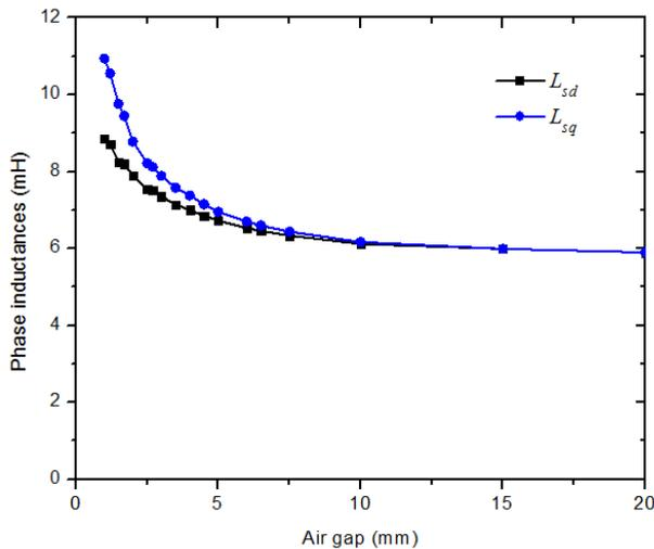
Fig. 7. Relation between phase inductance and air gap
