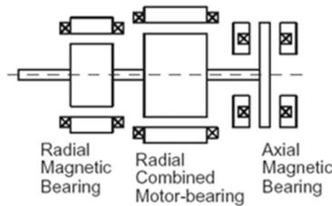
Fig. 2. Structure of radial-combined magnetic-bearing motor
