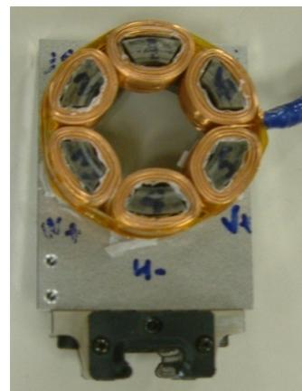
Fig. 16. Picture of the stator of the AGBM
