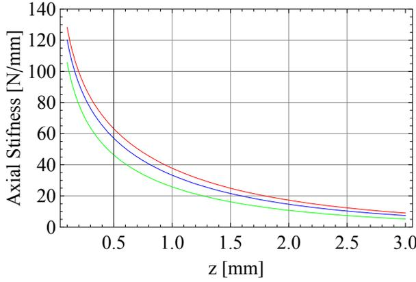
Fig. 18. Axial stiffness when the plane air gap length,  $z$ , varies.  $r_1 = r_3 = 25\text{mm}$ ,  $r_2 = r_4 = 28\text{mm}$ . Blue:  $h = 3\text{mm}$ , Green:  $h = 2\text{mm}$ , Red:  $h = 4\text{mm}$ .
