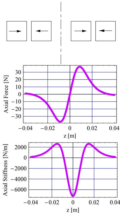
Fig. 22. Axial force and stiffness versus axial displacement for two ring permanent magnets with radial polarizations;  $r_1 = 0.01$  m,  $r_2 = 0.02$  m,  $r_3 = 0.03$  m,  $r_4 = 0.04$  m,  $z_2 - z_1 = z_4 - z_3 = 0.1$  m,  $J = 1$  T
