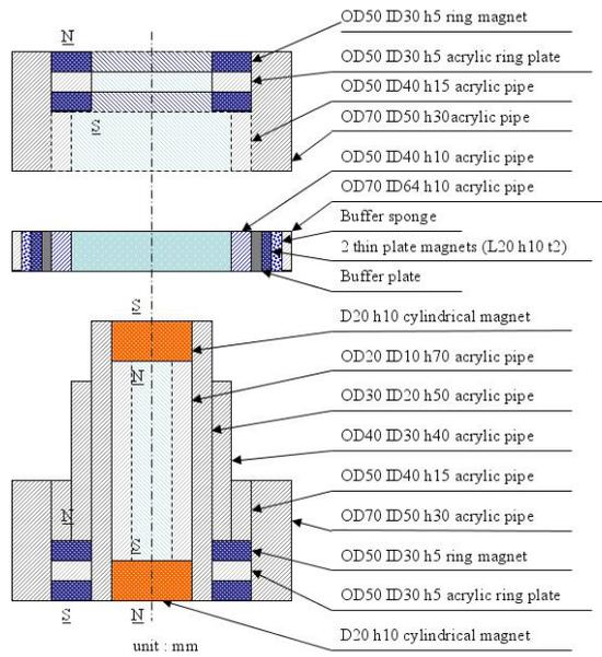
Fig. 3. Detail of component of the rotor model
