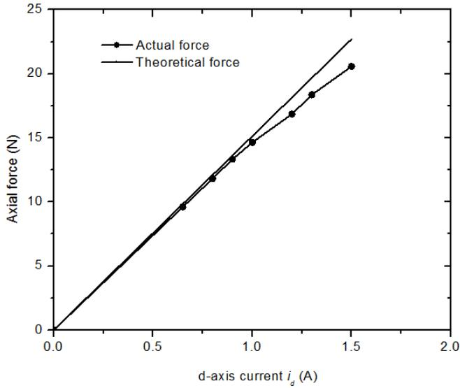
Fig. 8. Relation between axial force and d-axis current
