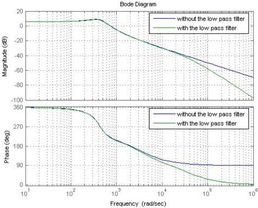
Fig. 5. Bode plot of the magnetic bearing system (a reduced 2<sup>nd</sup>-order model is used here) with the designed lead compensator
