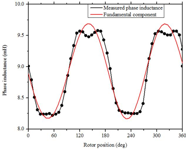
Fig. 6. Relation between phase inductance and rotor position
