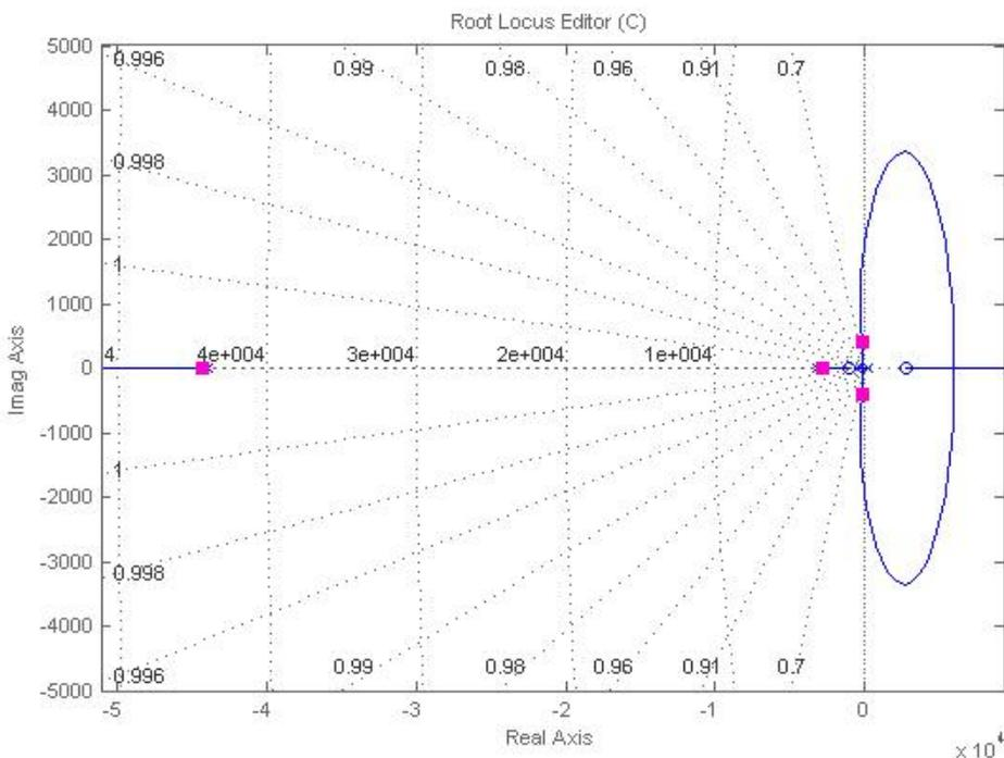
Fig. 4. Root locus of the magnetic bearing system (a reduced 2<sup>nd</sup>-order model is used here) with the designed lead compensator
