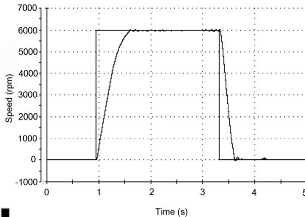
Fig. 18. Response of speed at zero displacement
