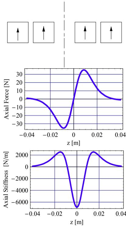
Fig. 23. Axial force and stiffness versus axial displacement for two ring permanent magnets with axial polarizations;  $r_1 = 0.01$  m,  $r_2 = 0.02$  m,  $r_3 = 0.03$  m,  $r_4 = 0.04$  m,  $z_2 - z_1 = z_4 - z_3 = 0.1$  m,  $J = 1$  T
