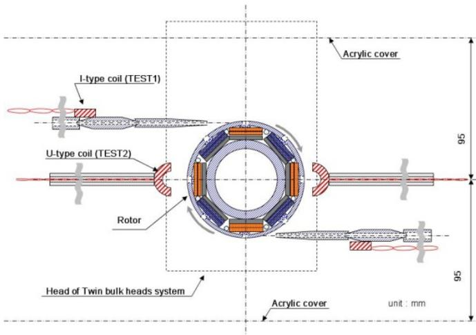
Fig. 10. Schematic drawing of the rotary mechanism part
