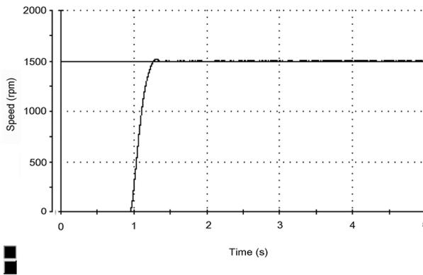
Fig. 19. Response of speed at start
