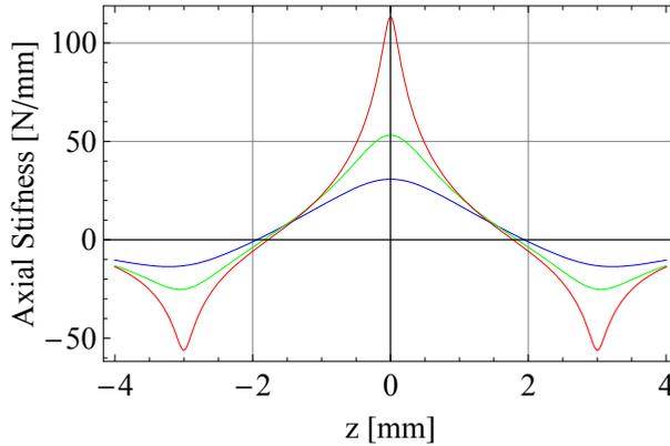
Fig. 4. Axial stiffness for several air gap radial dimensions. Blue:  $r_1 = 25\text{mm}, r_2 = 28\text{mm}, r_3 = 21\text{mm}, r_4 = 24\text{mm}, h = 3\text{mm}$  Air gap  $1\text{mm}$ , Green: Air gap  $0.5\text{mm}$ , Red: Air gap  $0.1\text{mm}$
