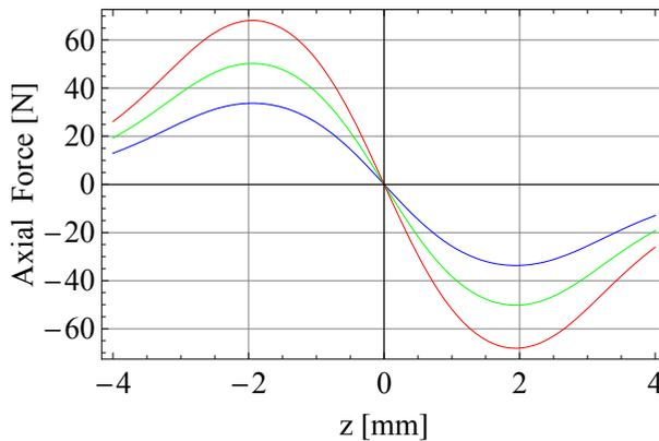
Fig. 9. Axial force for several air gap perimeters.  $h = 3\text{mm}$ , air gap  $1\text{mm}$ . Blue:  $r_1 = 25\text{mm}, r_2 = 28\text{mm}, r_3 = 21\text{mm}, r_4 = 24\text{mm}$ . Green:  $r_1 = 37\text{mm}, r_2 = 40\text{mm}, r_3 = 33\text{mm}, r_4 = 36\text{mm}$ . Red:  $r_1 = 50\text{mm}, r_2 = 53\text{mm}, r_3 = 46\text{mm}, r_4 = 49\text{mm}$ .
