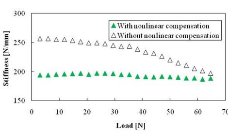
Fig. 8. Nonlinear compensation of the conventional zero-power controlled magnetic levitation system
