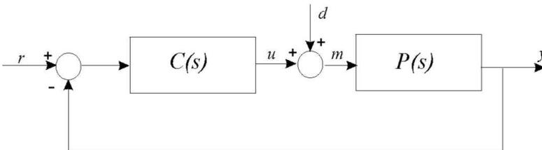
Fig. 3. A single-loop unity-feedback control system
