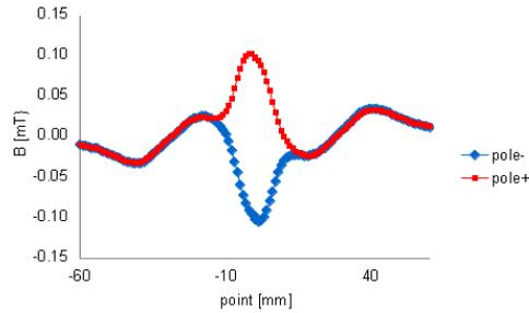
Fig. 6. Magnetic flux density of a rotary mechanism part of the rotor model
