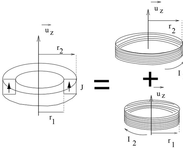
Fig. 2. Model of a ring magnet: amperian equivalence.
