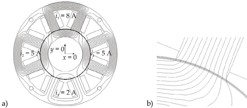
Fig. 5. Magnetic field distribution for the case  $i_x = 0$  A,  $i_y = 3$  A,  $I_0 = 5$  A, and  $x = y = 0$  mm; equipotential plot for the whole geometry (a), and in the air gap and the pole (b)
