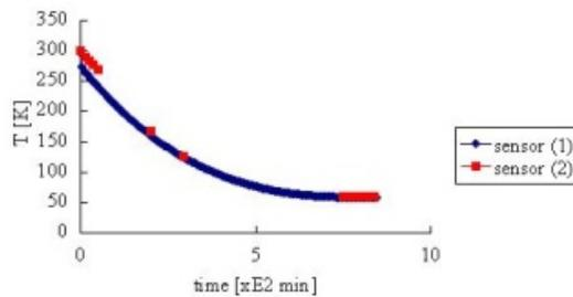
Fig. 8. The relationship between temperature of the cycocooler and time
