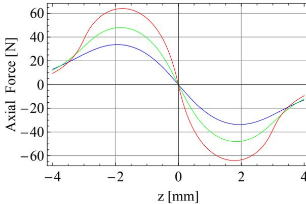
Fig. 3. Axial force for several air gap radial dimensions. Blue:  $r_1 = 25\text{mm}, r_2 = 28\text{mm}, r_3 = 21\text{mm}, r_4 = 24\text{mm}, h = 3\text{mm}$  Air gap 1mm, Green: Air gap 0.5mm, Red: Air gap 0.1mm
