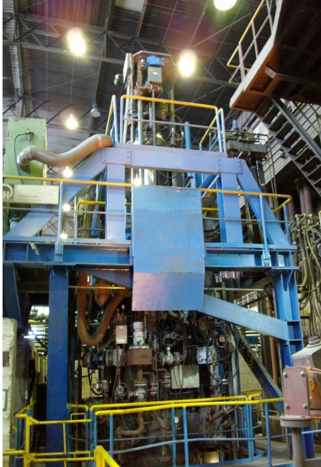
Fig. 3. View of the industrialized PESR –process at Energietechnik Essen GmbH for ingot weight up to 20 t und Ø1030 mm.
