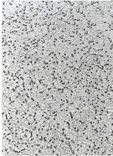
Fig. 5. Tempered microstructure of a nitrogen alloy martensite (1.4108). (M 1000:1)
