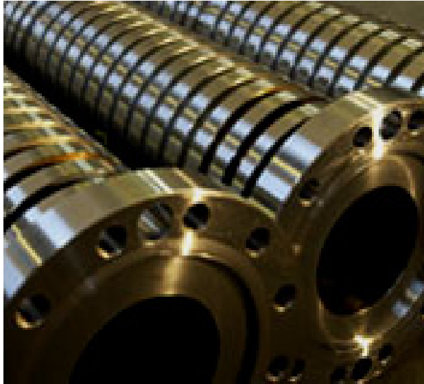
Fig. 25. Extruder screw, Cronidur 30 [ETE-11].
