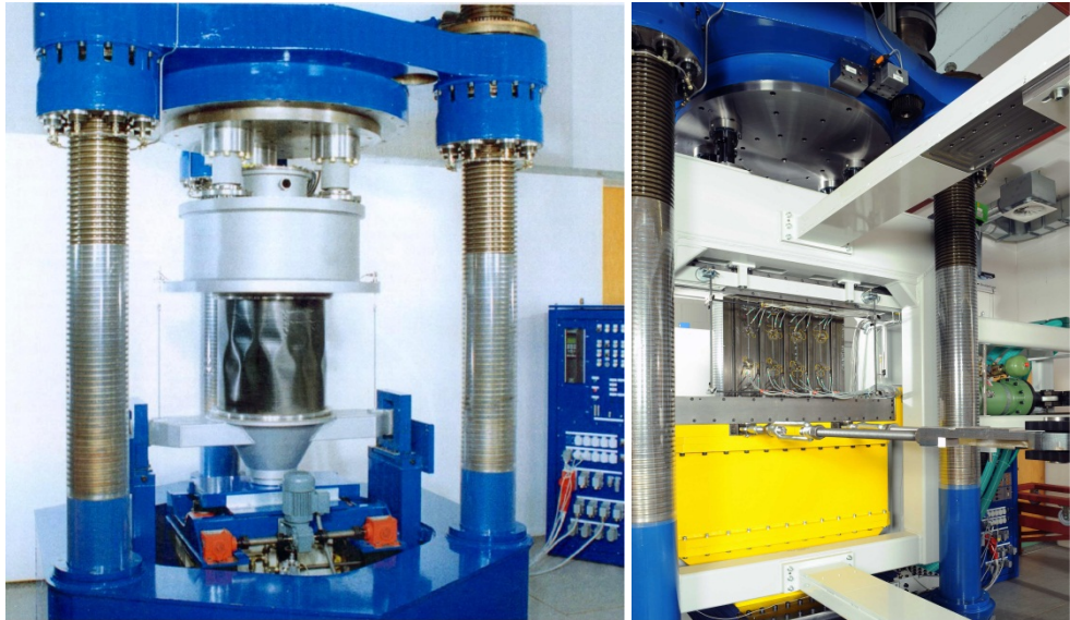
Figure 7. DLR's buckling test facility, axial compression configuration (left), compression-shear-configuration (right)
