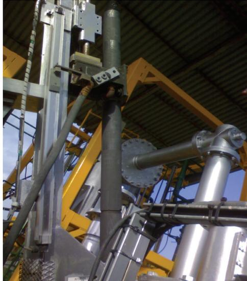
Photo 9. Movement Mechanism of the graphite electrode
