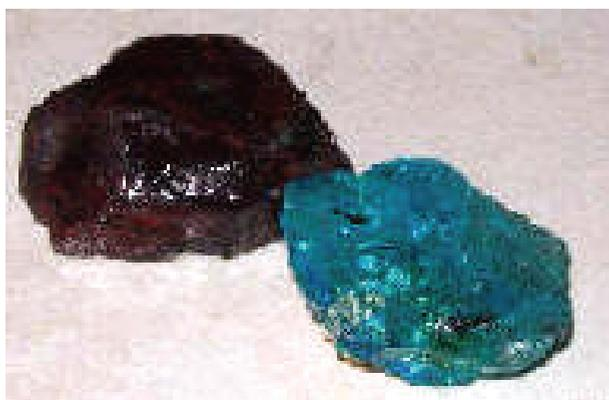
Fig. 10. Vitrified contaminants aspect after PPV reaction (<http://paginas.fe.up.pt/~jotace/gtresiduos/plasmapirolise.htm>).
