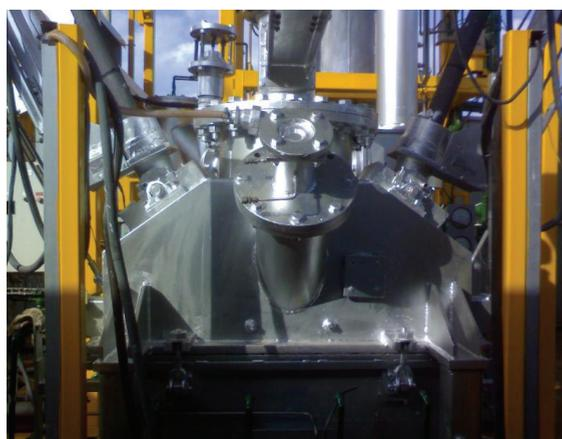
Photo 7. Gasification / vitrification furnace
