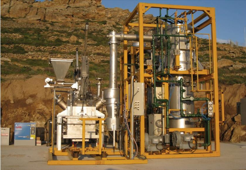
Photo 4. General view of the demonstration gasification / vitrification unit
