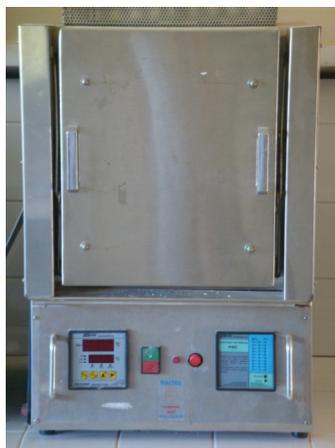
Fig. 3. Conventional oven used in the burning of the specimens
