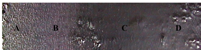
Fig. 4. Top view of the recrystallized silicon film, with increase of applied energy density from the left to the right
