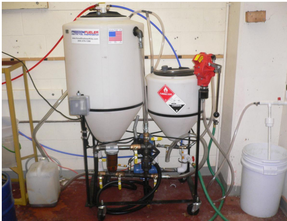
Fig. 3. Biodiesel Processor with a capacity of 40 gallons/day
