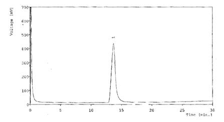
Fig. 1. GC of standard ricinoleic acid methyl ester
