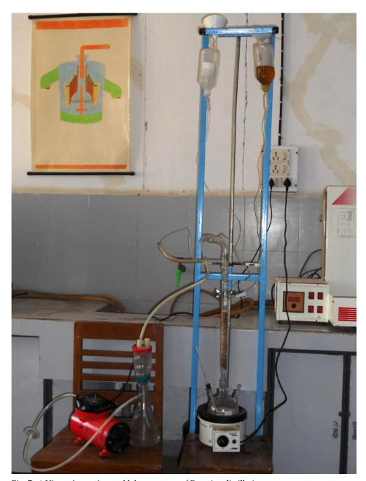
Fig. 7. a) View of experimental lab apparatus of Reactive distillation
