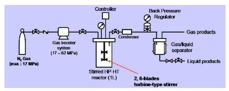
Fig. 1. Schematic diagram of batch-wise extraction system.
