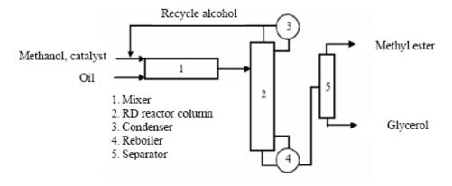
Fig. 5. Schematic of Reactive distillation column for biodiesel
