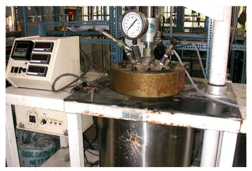
Fig. 3. Bench Scale lab Parr Reactor
