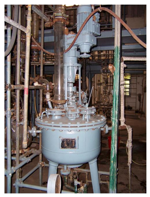
Fig. 5. (b) Pilot Plant scale reactor
