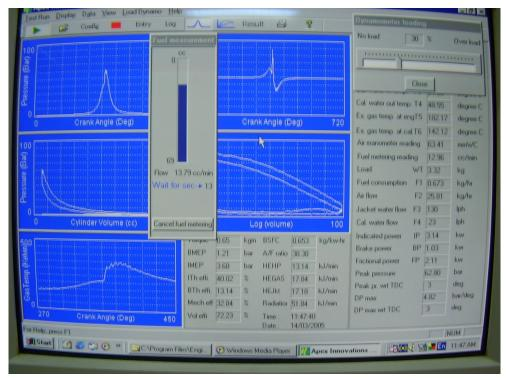
Fig. 10. Engine Calibration with "Engine-Soft"
