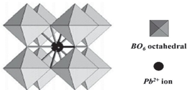
Fig. 10. Illustration of ideal ABO_3 -type perovskite structure, which can be described as a network of corner-linked octahedral.
