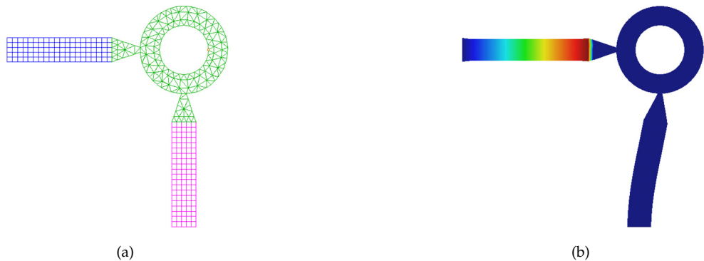
Fig. 16. Piezoelectric revolving drive: (a) FE grid; (b) Strongly scaled (factor of about 150) mechanical deformation for a characteristic time step, when the left actuator is at maximal load.
