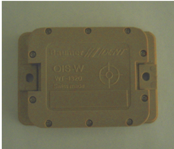
Fig. 12. SAW transponder used in automotive paint shops (Source: Baumer Ident).
