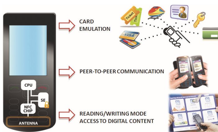
Fig. 1. NFC communication modes
