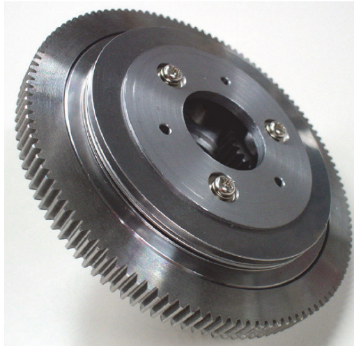
Fig. 5. Planetary gear produced in Hori laboratory
