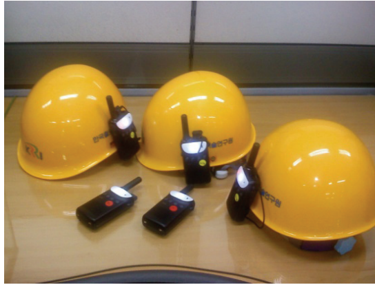
Fig. 17. Result of the prototype safety helmet for railways with bone conduction method
