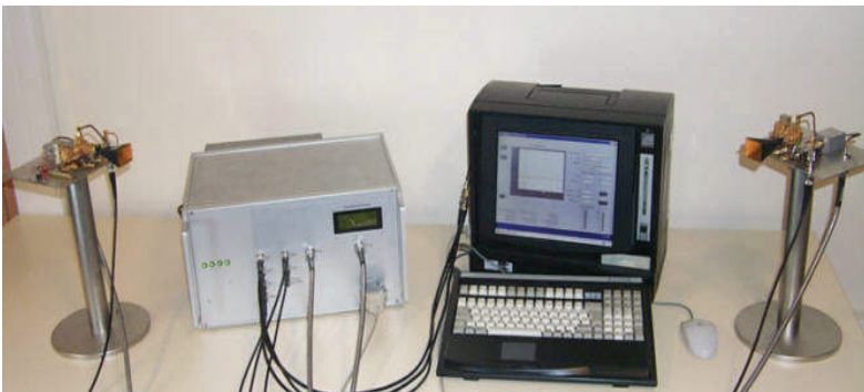
Fig. 1. Channel sounder at 60 GHz realized by IETR
