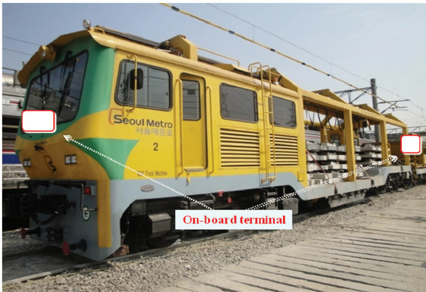
Fig. 14. Motor-car having a long length where 2 sets of on-board equipment were installed
