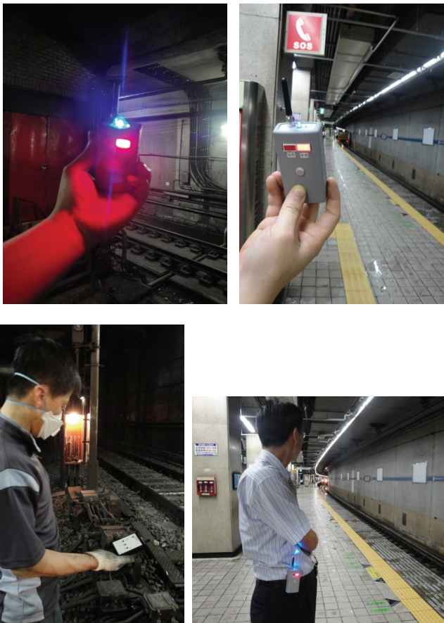
Fig. 13. Picture of the field test for worker terminal
