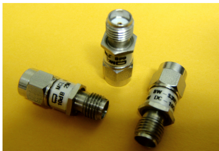
Fig. 14. Photograph of the 3, 6 and 10 dB coaxial attenuators.
