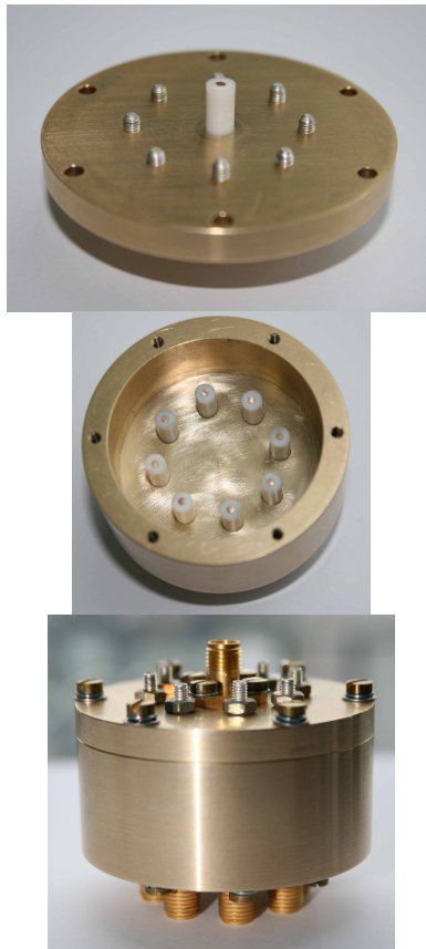
Fig. 14. Manufactured model structure of nine-port power splitter/combiner
