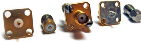
Fig. 18. Measurement kit: a panel SMA connector, a measurement probe, open, short and matched ( 50\ \Omega ) load calibration standards
