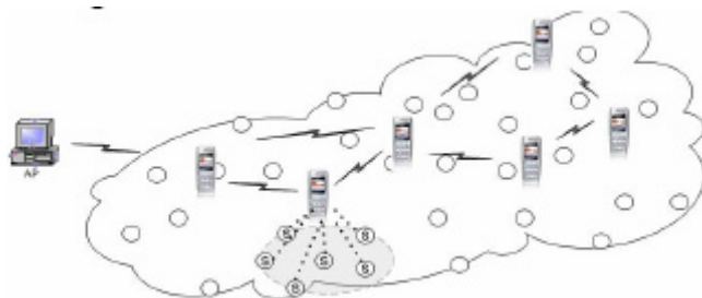
Fig. 4. Two-Tiered Sensor Network with Ad Hoc Configuration
