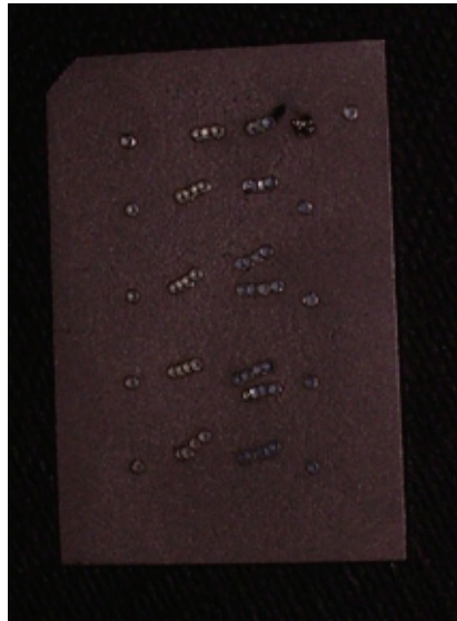
Fig. 3. The CrCoMo plate shot with different parameters.
