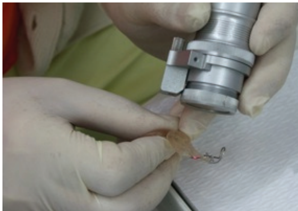
Fig. 25. Laser welding process without filler metal
