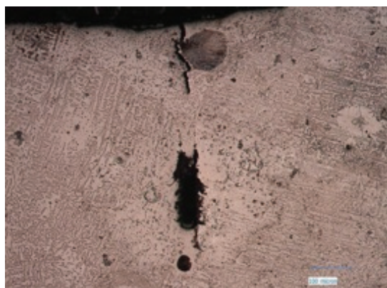
Fig. 12. Sample of laser welding by Rofin without filler chemically attacked
