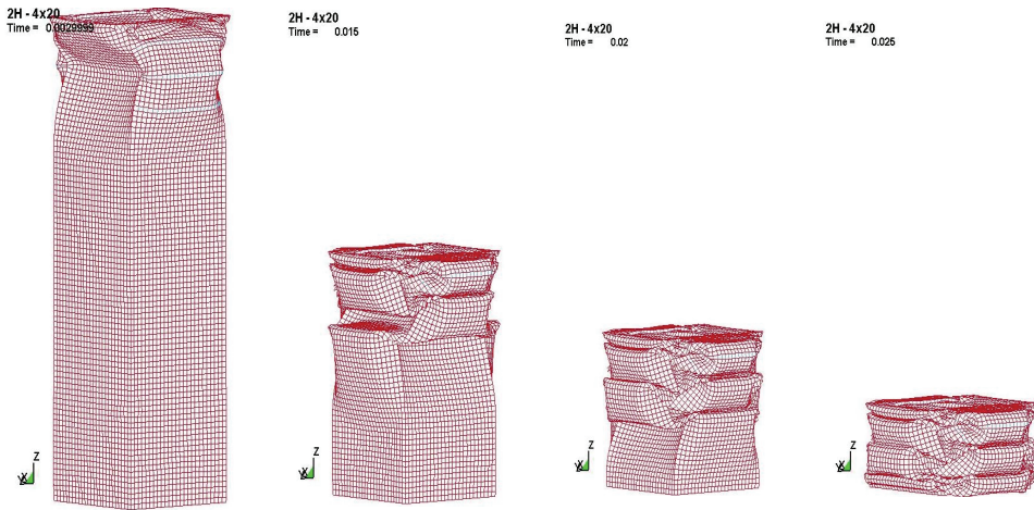
Fig. 26. Deformed shape along of the model (4x20) with 3mm width of the four HAZ triggers.
