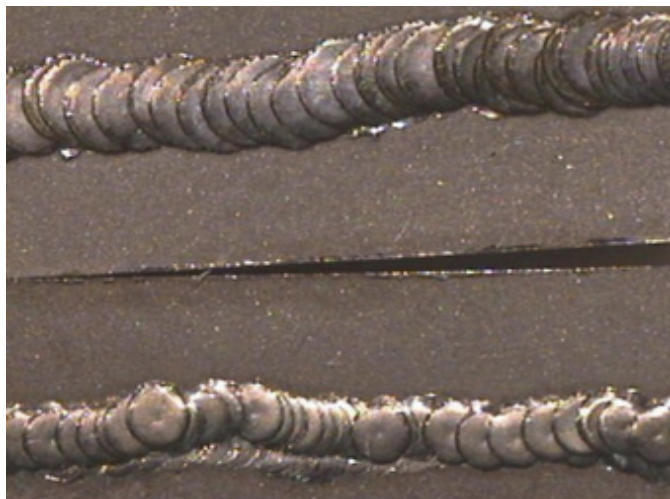
Fig. 6. Comparison between office and laboratory laser welding beads
