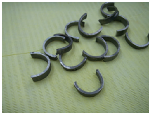
Fig. 21. Metallic plates in ARGELOY NP SPECIAL curved to hemispherical shape
