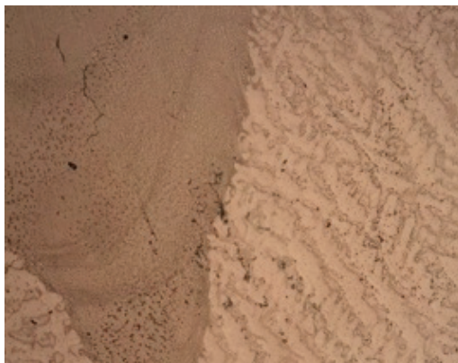
Fig. 13. Sample of laser welding by Fidelis with filler chemically attacked
