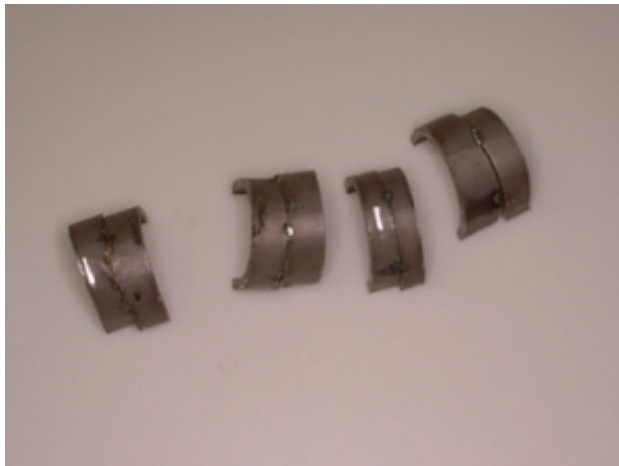
Fig. 23. Metallic plates welded, by Nd:YAG Laser, in three points (occlusal, vestibular and lingual).
