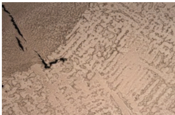
Fig. 11. Sample of laser welding by Fidelis without filler chemically attacked
