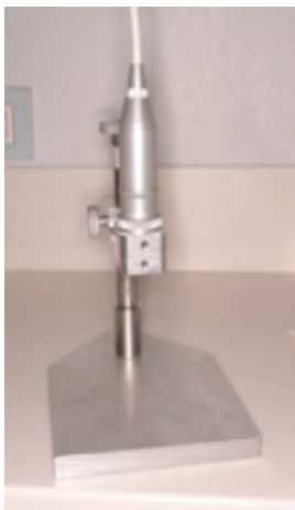
Fig. 2. The metallic support used in order to put firmly handpiece
