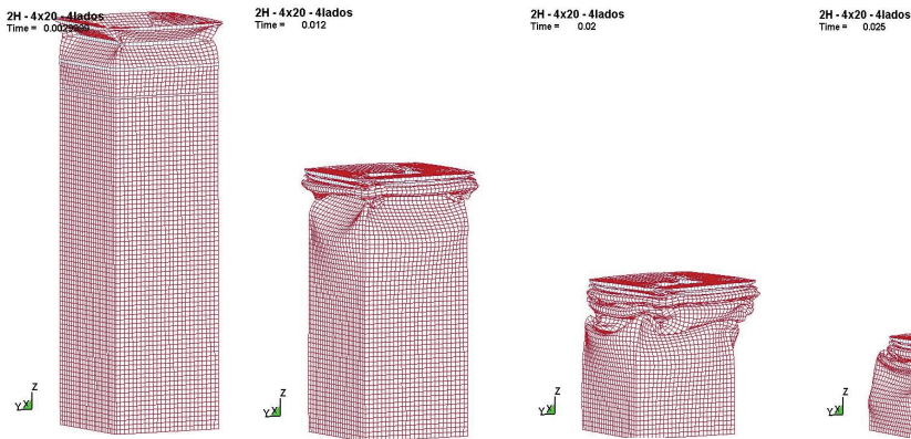
Fig. 27. Deformed shape on model with four HAZ triggers around the model with 3mm width (4sides 4x20).
