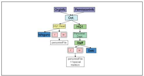
Fig. 4.4-3 Data structure of the image by "OrgInfo×(HQ1×Oct.)+PermissionInfo×(r+w)×person nelFile"
