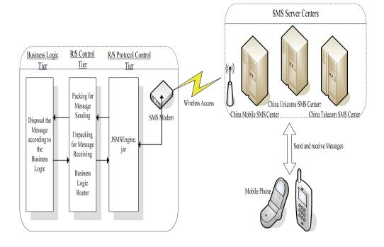
Fig. 8. the model of GSM-Modem
