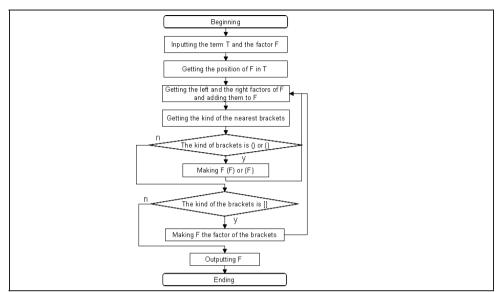
Fig. 4.2 The flowchart of the algorithm for a quotien
