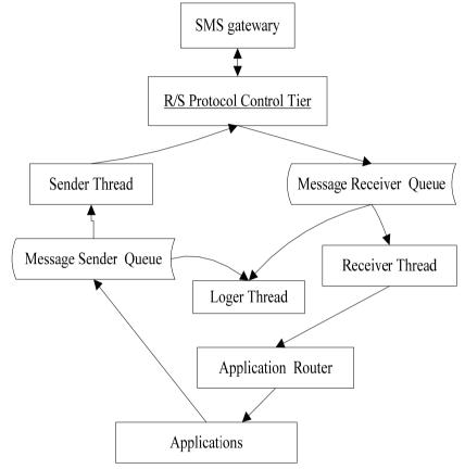
Fig. 9.Structure of the R/S Control Tier
