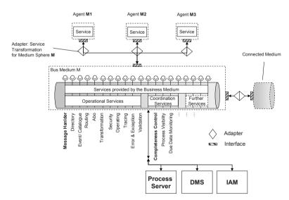
Fig. 13. Technical view: the HERA-bus and its core constituents (Streit et al., 2009)
