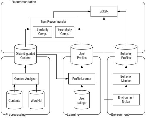
Fig. 1. General system architecture
