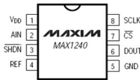
Fig. 9. MAX1240 pin distribution
