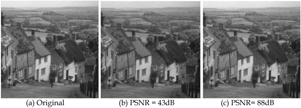
Fig. 7. (a) Original goldhill image; (b) Reconstructed image using FP scheme (8-bits); (c) AIQ scheme (14-bits).
