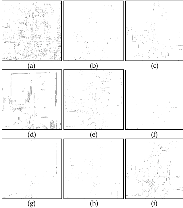
Fig. 24. (a) Noise edges. (b) Ramp edges. (c) Step edges. (d) Pulse edges. (e) Stair edges. (f) Ridge edges. (g) Roof edges. (h) First non-antisymmetrical step edges. (i) Second non-antisymmetrical step edges.
