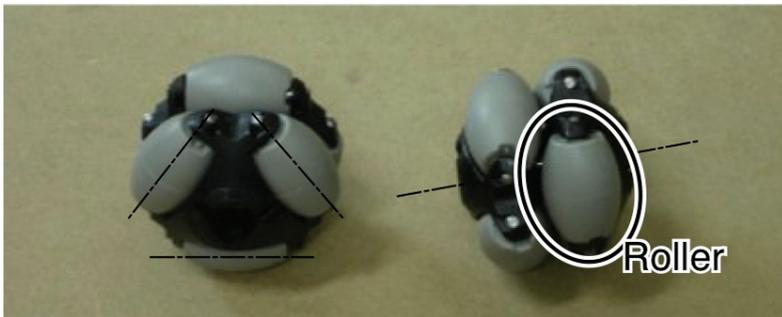
Fig. 6. Omnidirectional Wheel
