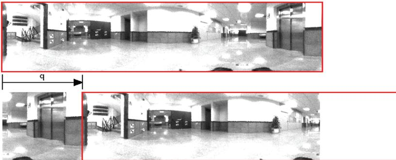
Fig. 3. Two panoramic images captured in the same point of the environment but with different heading for the robot.
