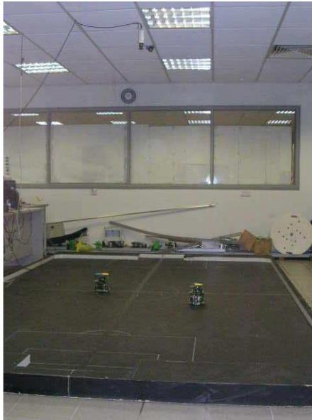
Fig. 8. Picture of real robots, test bed(on the floor), CCD color camera with wide-angle lens and one web-cam (mounted on the ceiling).
