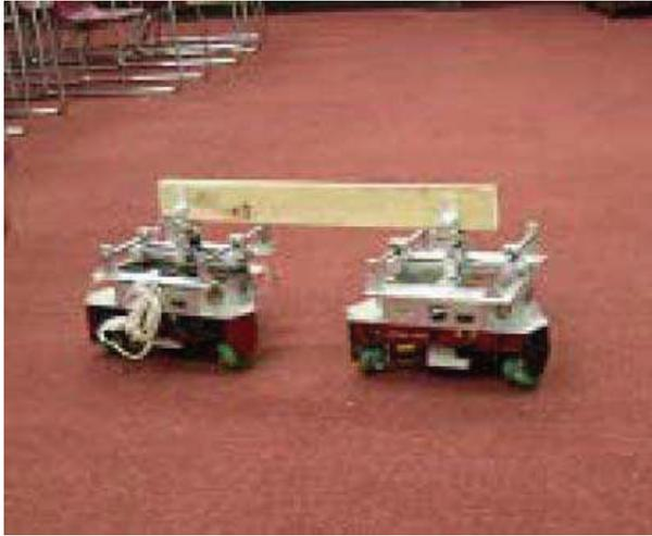
Fig. 5. Omni-wheeled robots utilized for experimentation
