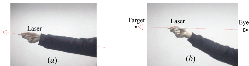
Fig. 3. (a) The laser pointer was used to represent the arm's direction (b) The laser pointer used with the line-up method, where the target, two ends of the laser pointer and eye are collinear.
