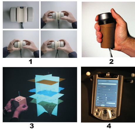
Fig. 4.1. Selected interaction devices developed in the Virtual Environments department of Fraunhofer IAIS (1 – YoYo, 2 – NoYo, 3 – CubicMouse, 4 – PioDA)
