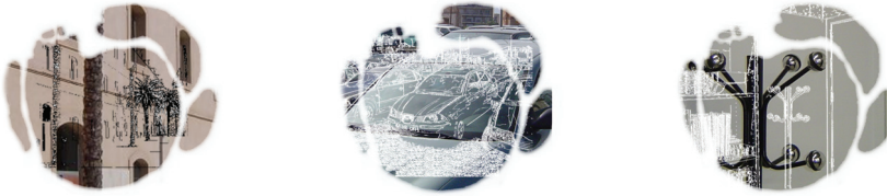
Fig. 4. Simulation of patient's view through the HMD for outdoor and indoor environments. A residual 10^\circ field of view has been considered to simulate the tunnel vision effect.
