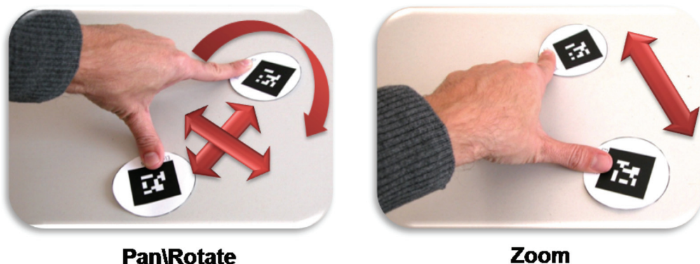
Fig. 3. Tangible interface model navigation using two paper markers
