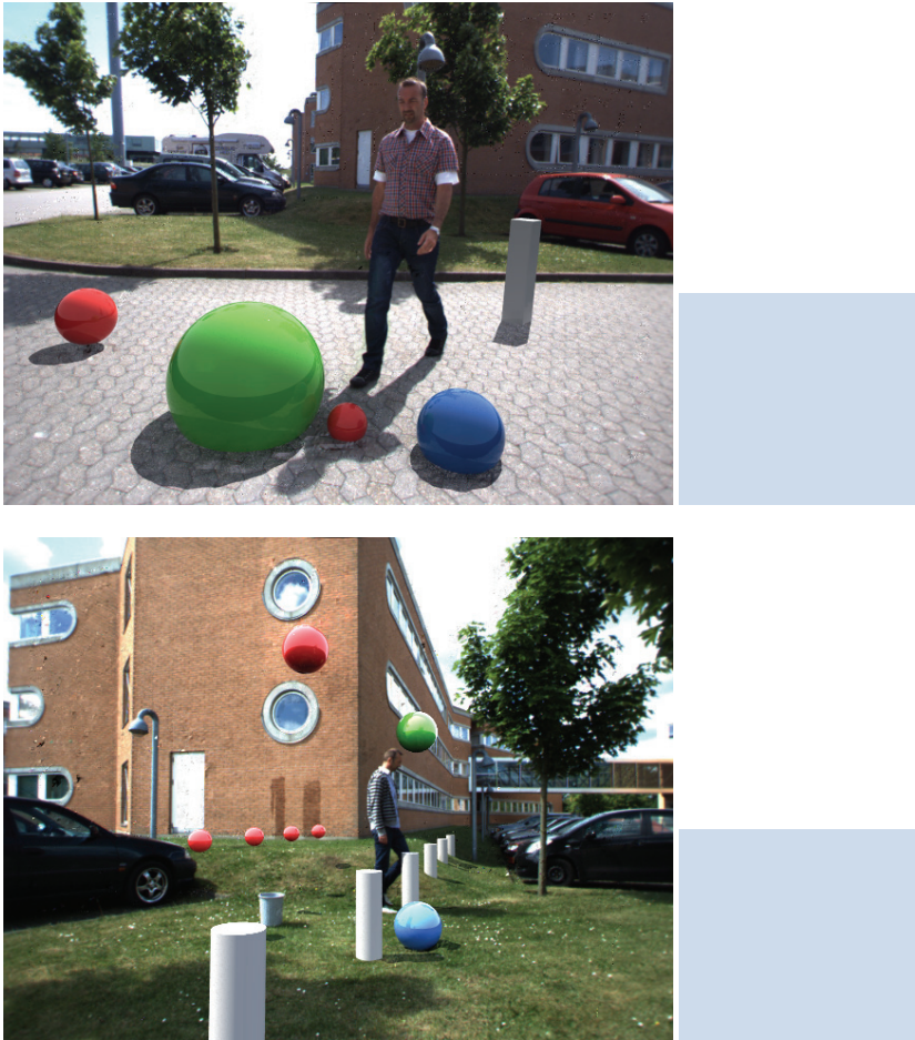
Fig. 10. Two different augmented scenes. The small blue fields on the right are the estimated sky colors (the color balance estimated for the sky using the presented technique).
