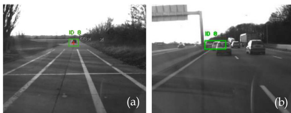
Fig. 11. (a): Detection from optical identification system projected in the right image. (b): Error in detection: ID lamp reflected on the road separating wall. This error is correctly discarded by the stereovision-based validation step.
