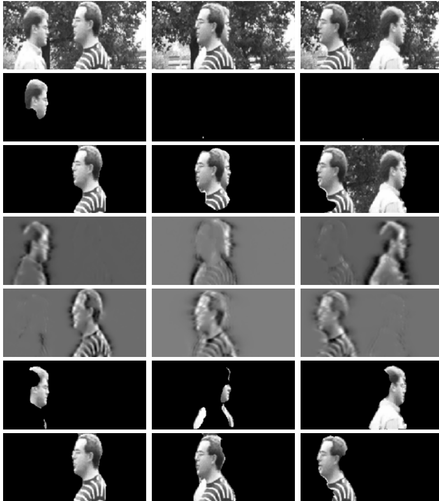
Fig. 13. Three frames of a sequence showing two occluding motion patterns. 1st row: Input data. 2nd and 3rd rows: Inter-frame difference based segmentation, using a different initialization for each of the motion patterns. 4th and 5th rows: \Psi_{\text{even}} of two of the obtained composite-features, corresponding to the two motion patterns. 6th and 7th rows: Segmentations produced using composite-features from rows 4th and 5th respectively.
