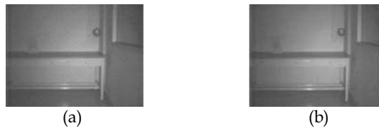
Figure 8. (a) Input low light-level image with significant noise and (b) NAST filtered image
