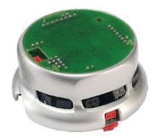
Fig. 2. The miniature mobile robot: Khepera
