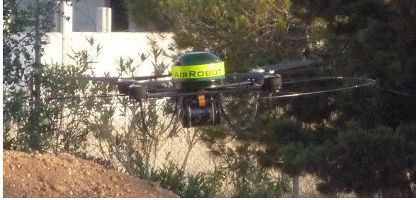
Fig. 4. The AR-100 UAV with the camera mounted beneath the flight board.
