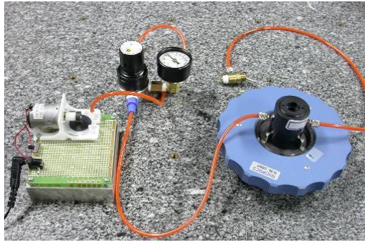
Fig. 3. Soft zoom lens system contain pneumatic supply device for control unit.
