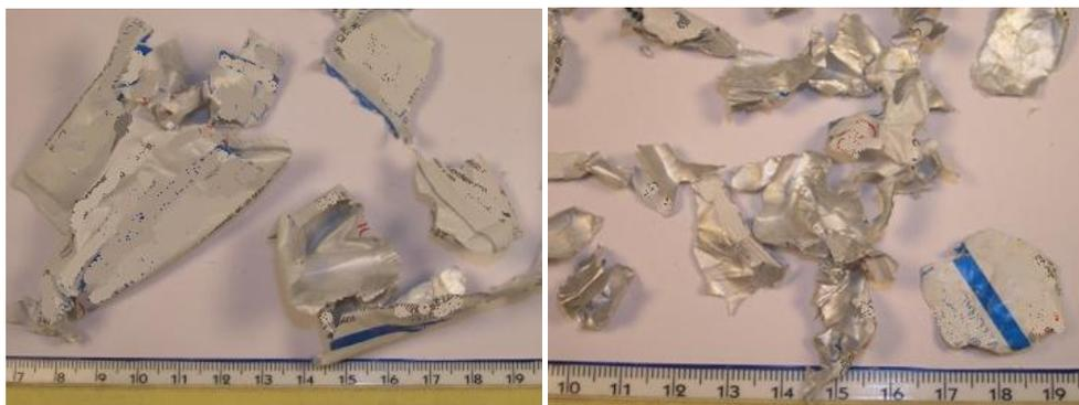
Fig. 9. Comminuted flexible multi-layered sachets containing granular medicine, belonging to the size class  $+1.0$  mm, obtained in the preliminary tests without control grid (left) and with 20 mm mesh control grid (right).
