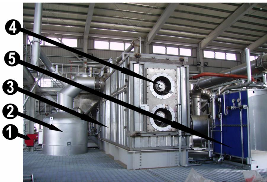
Pict. 1. ENRESTEC thermal units for waste tire pyrolysis with steam: 1 – oil fuel burner, 2 – furnace, 3 – pyrolysis reactor heating box, 4 – double-screw reactor in the box, 5 – second heat steam boiler.
