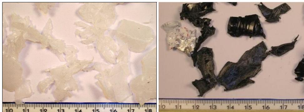
Fig. 7. Comminuted bottles in HDPE (left) and PET (right) obtained in the preliminary tests with the adoption of a 20 mm mesh control grid.
