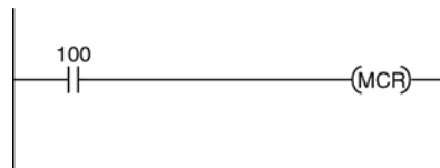
Figure 1.8 Master Control Relay
