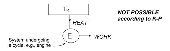
Recall, a reservoir is a body that has so much thermal capacity that its temperature doesn't change when heat transfer occurs
