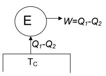
This engine takes heat from one reservoir  $(T_c)$  to produce work  $\rightarrow$  this is *not* possible according to K-P statement and thus demonstrating the equivalency of the two statements
