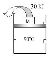
Engine consists of a frictionless, adiabatic piston-cylinder device with two sets of stops and weight placed on the piston. Initial temperature of the gas is 30°C
