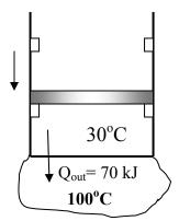
For 100% efficiency the 70 kJ excess energy added to the gas must be returned to the 100°C source for later use  $\rightarrow$  results in heat flow from cold to hot, *Clausius statement says not possible*
