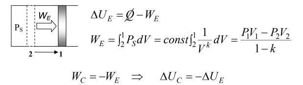
When the piston is returned to the initial position: 1) the system IE is recovered,  $\Delta U_{1-2} + \Delta U_{2-1} = 0$ 2) the energy from the surroundings used to compress the gas is returned by the work done by the gas during expansion
