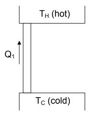
Connect two thermal reservoirs with high thermal conductivity metal and assume  $Q_1$  heat flows from  $T_C$  to  $T_H$  which according to Clausius is *not* possible
