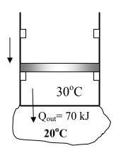
Must transfer heat to colder reservoir, say 20°C, to drop temperature back to 30°C 70 kJ excess energy rejected
